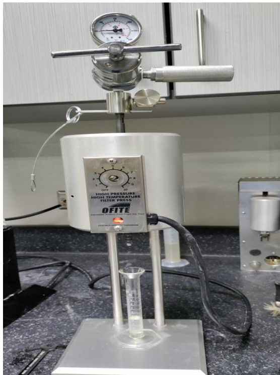
Figure 17. HPHT filter press with a measuring cylinder for collecting filtrate loss.
