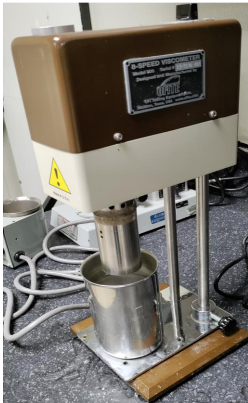
Figure 16. 8-Speed viscometer for measuring rheological properties.
