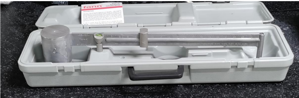
Figure 15. A Mud balance.
