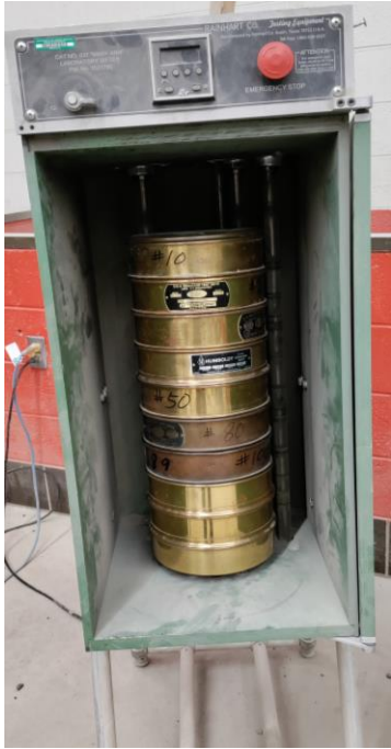
Figure 8. Stack of sieves with fly ash sample placed in a sieve shaker.
