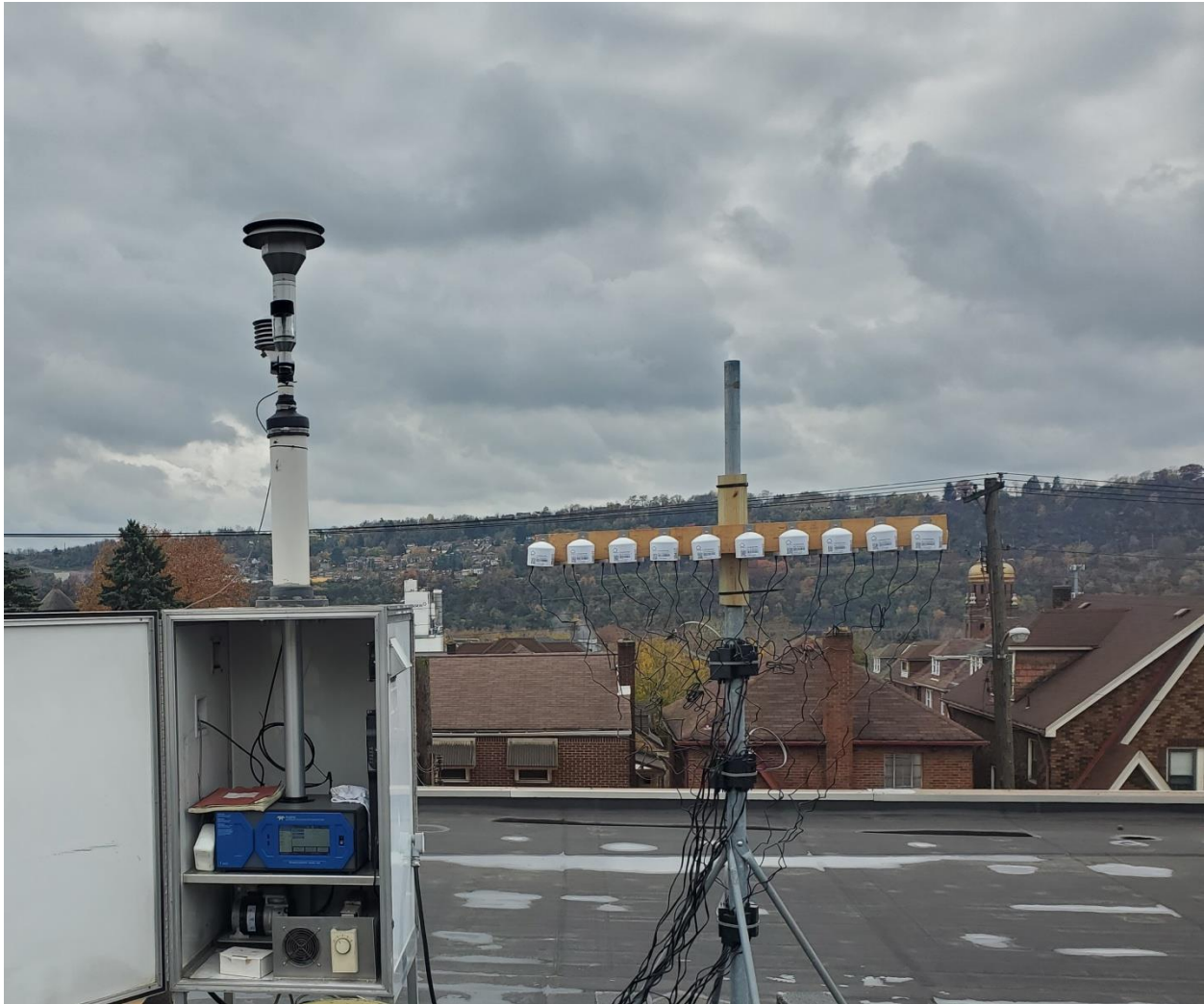
Figure 3.2. Air Sensor Collocated with Reference Instrument (T640) in North Braddock
