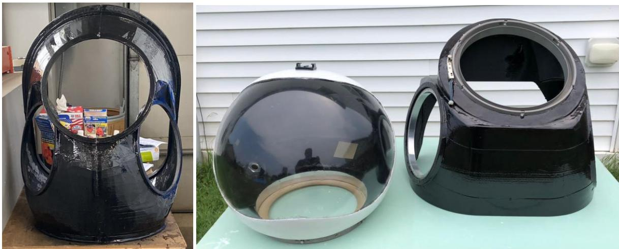
**Figure 5.3.1.-1. 3D Printed HUTs. [Left] custom sized NDX-4 HUT, featuring a rear entry hatch [Right] NDX-3 HUT, featuring a dual planar entry method**
