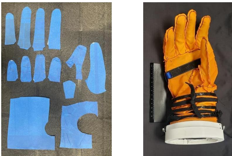
**Figure 1.8.-1. [Left] Glove Sewing Patterns [Right] Assembled Glove.**
