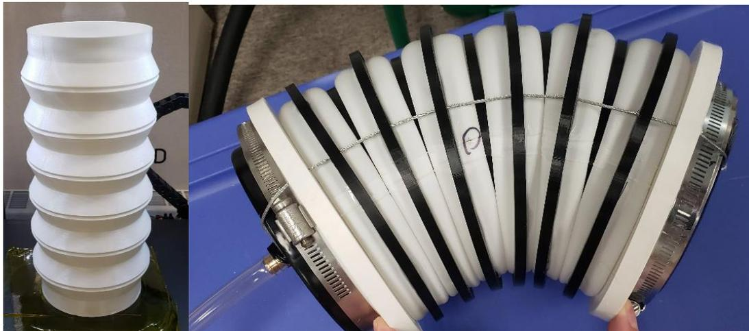
**Figure 5.2.7.-2. Bellows Assembly** [Left] flexible bellows component as [Right] assembled bellows assembly.
