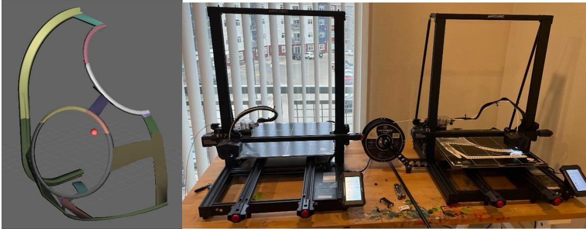
**Figure 5.2.-1. 3D Printed Mockup Process.** [Left] CAD geometry of skeletonized HUT mockup [Right] 3D Printers used to fabricate HUT mockups.
