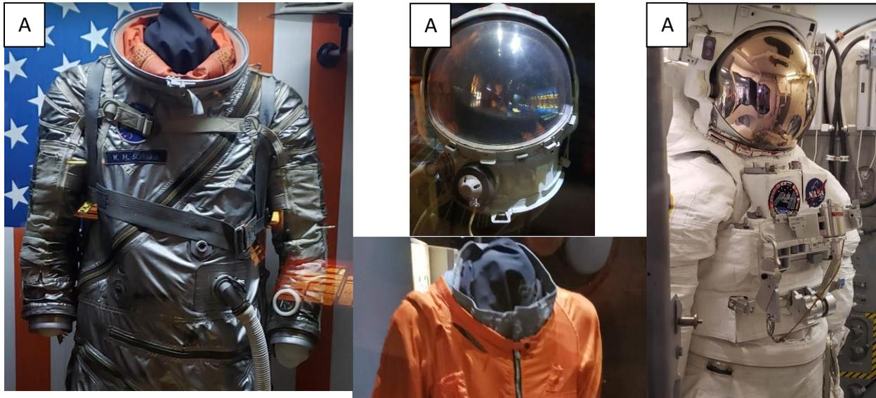
**Figure 1.3.2.-2. Alternative suit entry methods, [Left] Mercury spacesuit, with spiral zipper entry [Middle] SK-1 Soviet training spacesuit, with a neck entry method [Right] Shuttle EMU, with a waist entry method.**
