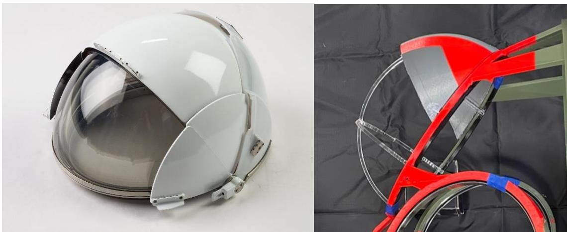
**Figure 2.4.4.-1. EVAAs A: xEMU EVVA prototype B: Mockup EVVA used for HITL testing of HUT mockups.**
