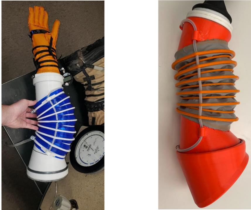
**Figure 5.2.4.-1. Spacesuit Arm Assembly Design Evolution.** [Left] 1<sup>st</sup> generation 3D printed spacesuit arm assembly [Right] 2<sup>nd</sup> generation 3D printed spacesuit arm assembly.
