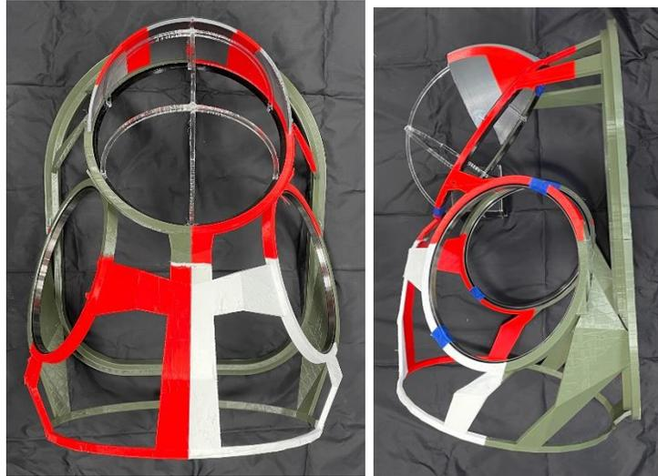
**Figure 2.4.-1. Skeletonized HUT Mockup with Additional Hardware Mockups and Bearings Installed.**
