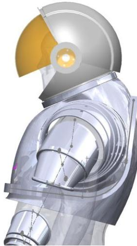
**Figure 6.1.-1. Conceptual Design of a Dual Planar 3D Printed Spacesuit**
