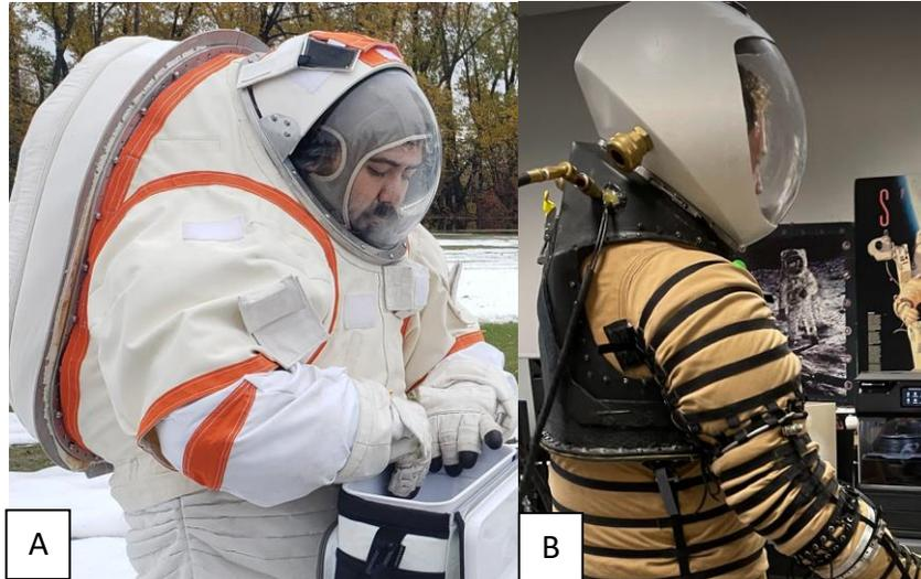
**Figure 1.3.1.-2. Effect of entry method on spacesuit torso shape, A: NDX-2AT, rear entry hatch spacesuit, B: NDX-1, dual planar spacesuit**
