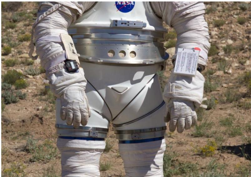
**Figure 1.6.2.-1. Waist-Brief-Hip Components of the Mark III EVA Spacesuit Prototype**
