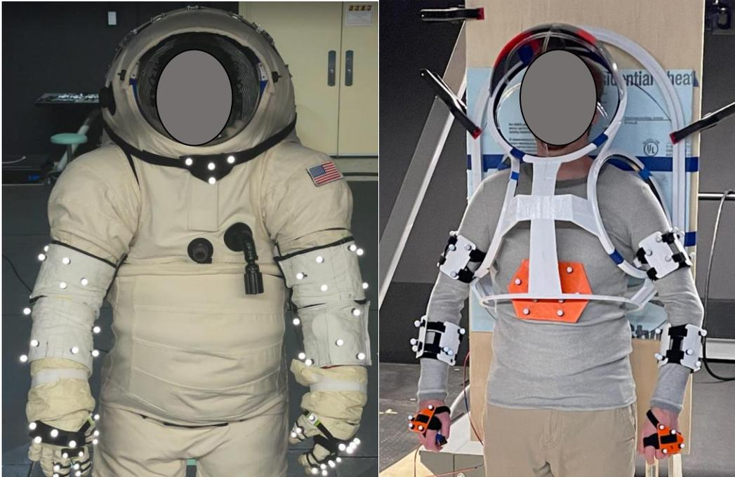
**Figure 4.2.1.-2. IR Motion Capture Tracker Plates.** [Left] suited tracker system [Right] shirt sleeve tracker system.
