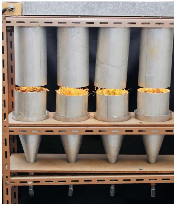
Figure 4. Berlese funnel used to separate invertebrates from soil samples.
