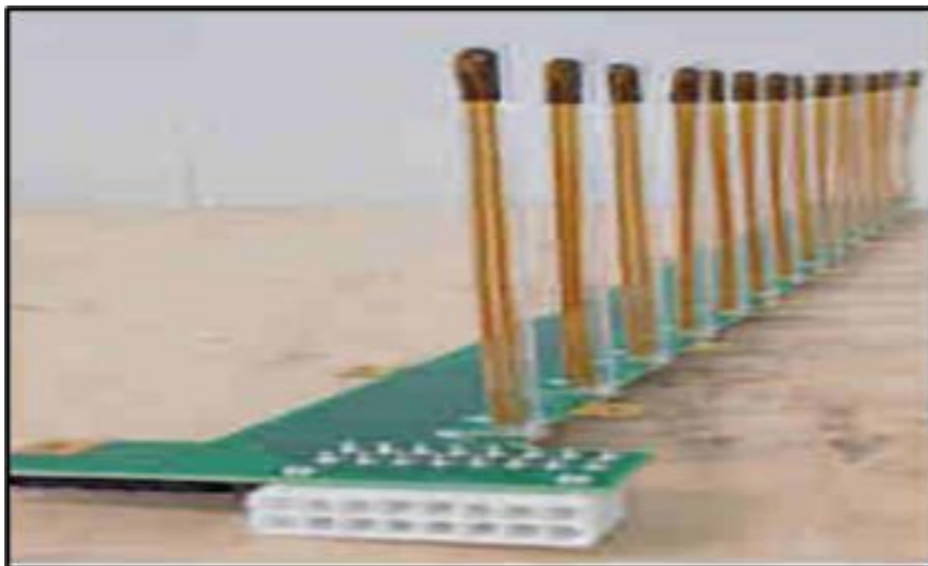
Figure.80 - A sub view image of the multiple temperature sensors for detecting temperature change in the lithium module structure.
