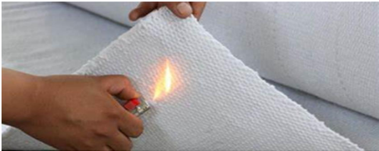
Figure.82 - An image of fire-retardant material to maintain stop fire propagation. Material test conducted by Daniel Kelly Boakye Danquah, 2021. Source: www.suntexfiberglassfabric.com
