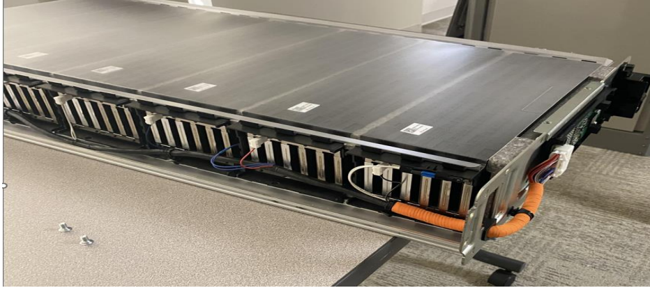
Figure 69 - Internal view of the lithium-ion battery with electronic board and sensors. Source: Produced by Daniel Kelly Danquah @LGEUS lab.2023.
