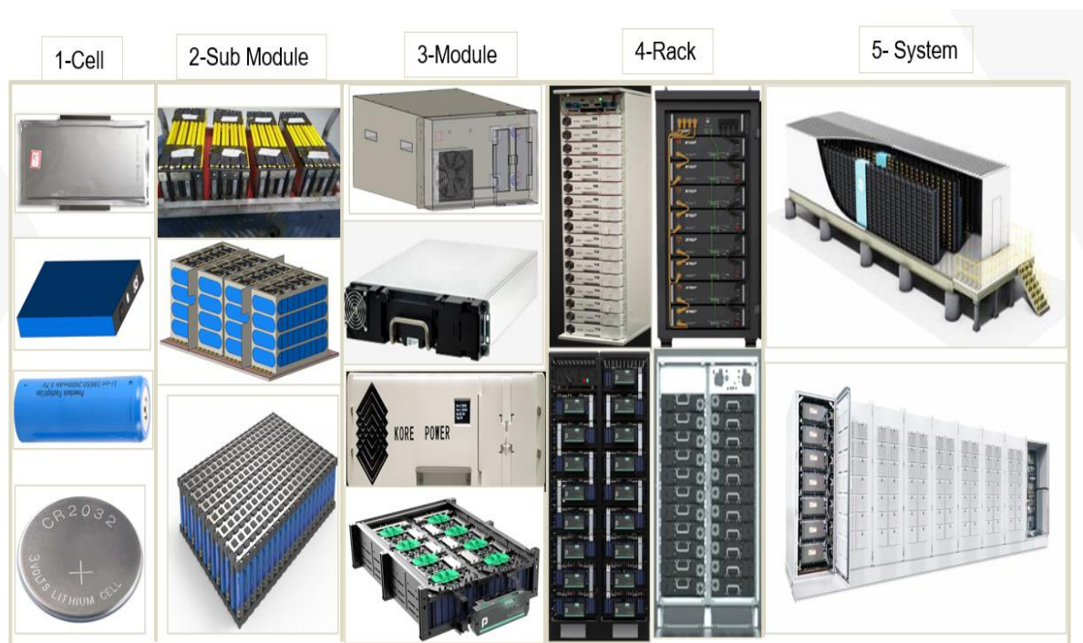
Figure 72 -Energy storage system architecture from cells, module, rack, and System Source: Daniel Kelly Boakye Danquah
