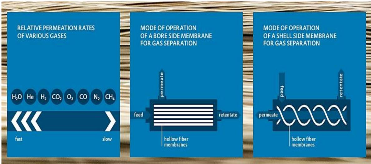
**Figure 7.24.** Helium selective hollow-fiber membrane operation. From Evonik, 2021.
