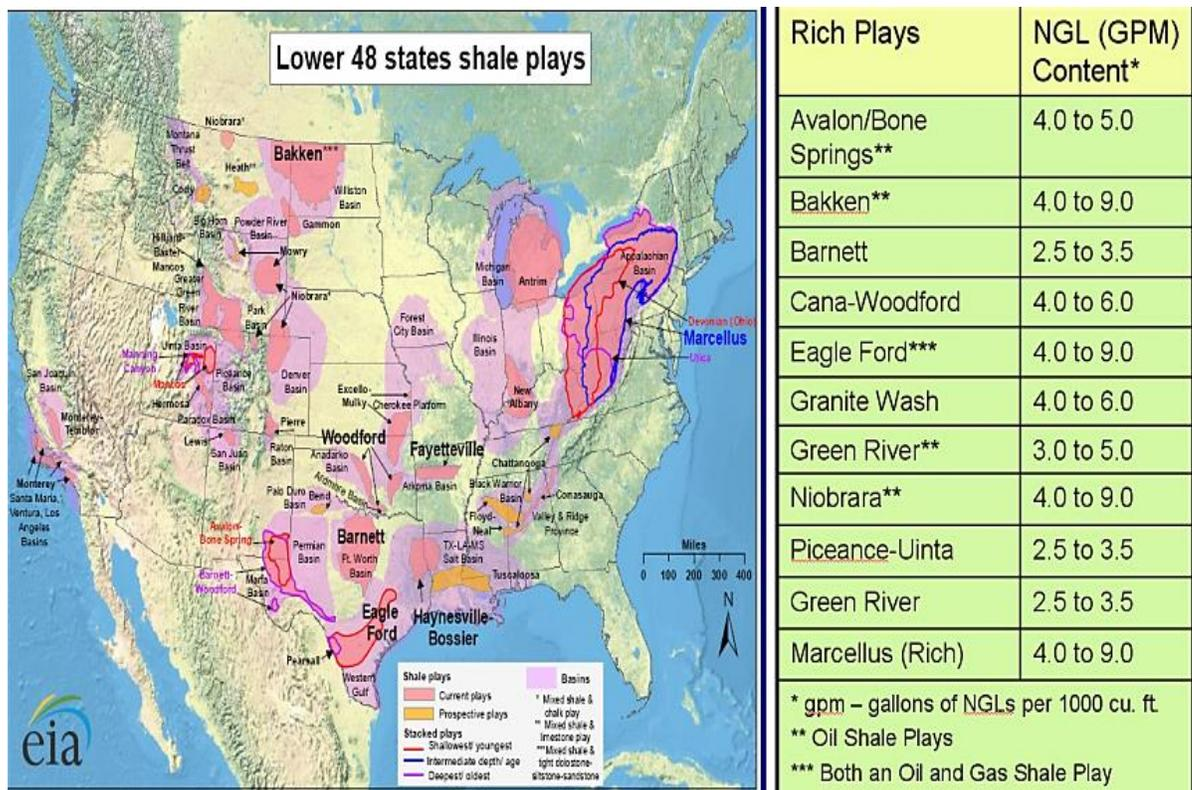
**Figure 7.18.** Natural gas liquids, processing economics. Note the GPM content for the Bakken. From Keller, 2012.
