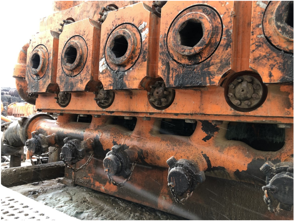
Figure D. 4 - Fluid end of a positive displacement frac pump. Photograph was taken in Wyoming.
