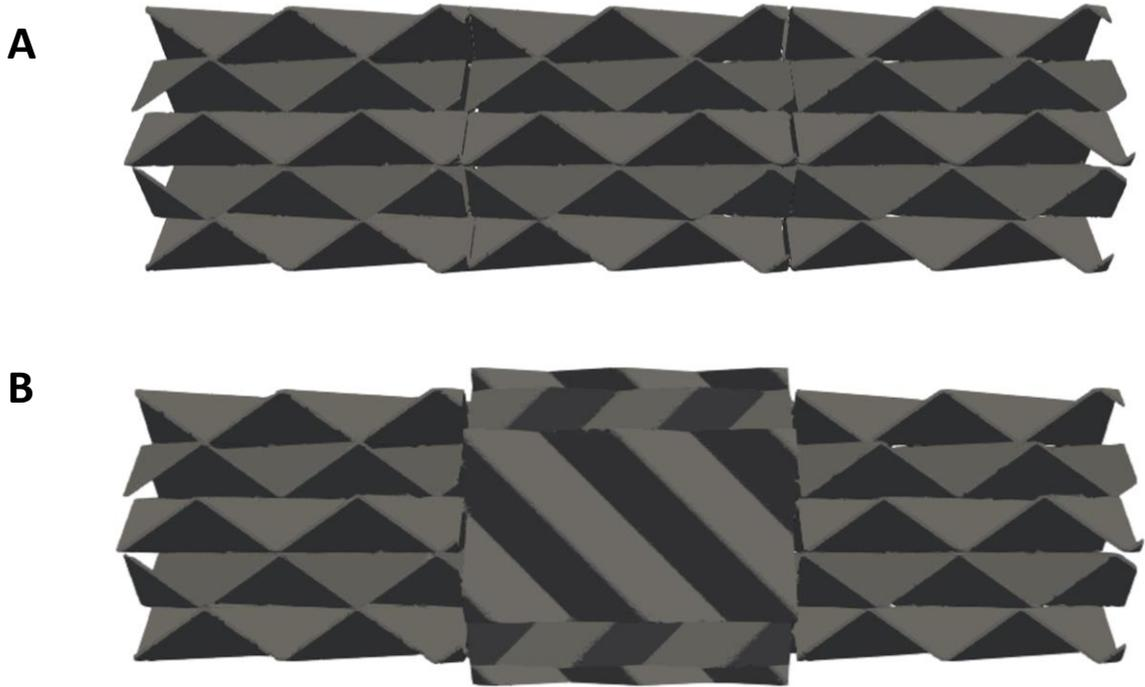
Figure 3.1. Aligned (A) and rotated (B) configurations with three mixing elements
