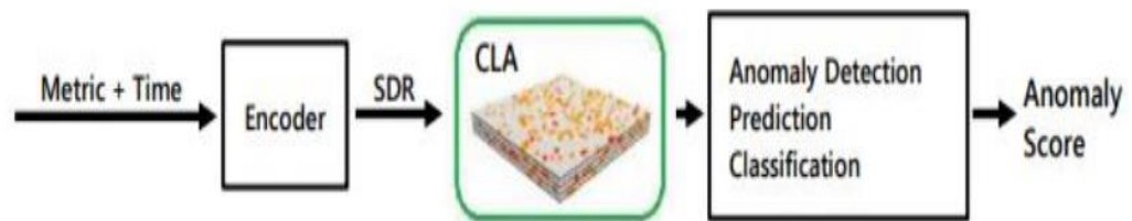
Figure 2.15 Block diagram for Applications using HTM High-Order Inference (Ahmad and Hawkins 2017)
