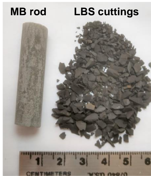
Fig. 7.5 Geometries of the rock samples used by Hawthorn et al. [111] for gas HnP experiments, 0.44 in diameter * 1.75 in length rods to represent the MB (left) and 0.04-0.13 in cuttings for the LBS (right)
