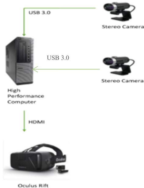
**Figure 3. 1. Overview of the prototype.**
