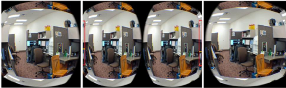
**Figure 4. 6. The results generated by the proposed model (Real + HMD + FOV model). The Oculus view of the left and right eyes - the right image is on the right and the left image is on the left, the image on the center is the generated image on the display Oculus. The red line with the yellow line shows the parallax rendered on the display. There is more parallax rendered compared to the previous model.**
