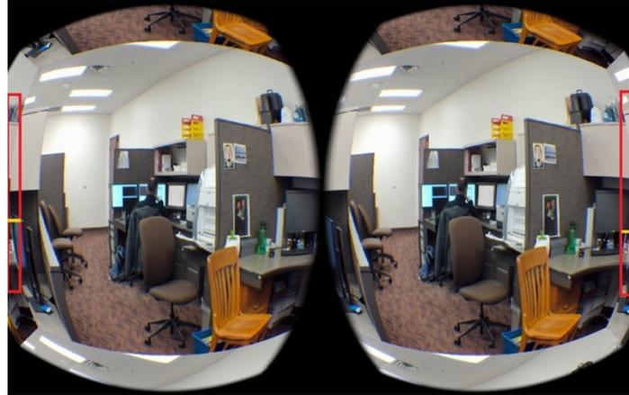
**Figure 4. 5. The Oculus view of the two rendered images on the two Oculus eyes - the red box shows the parallax which is more compared to figure 4.1.**
