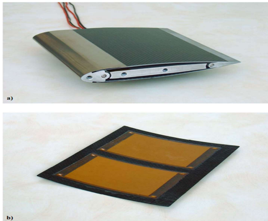
Fig 3.11 (c) (a) Prepared Materials for Model Aerofoil Built (b) aerofoil's inner skin with MFC [19]
