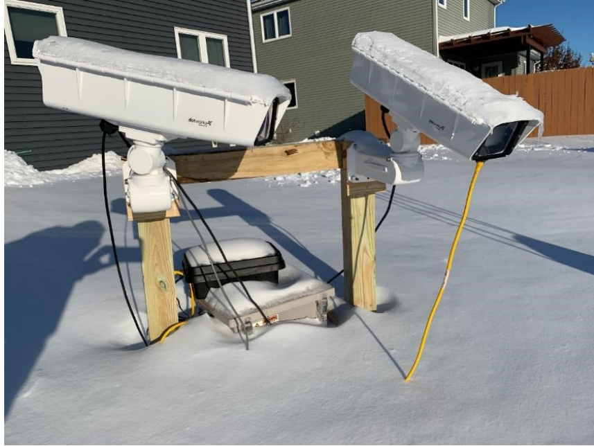
Figure 6 – A picture of the OSCRE. The camera (left housing) captures pictures of hydrometeors in its field of view at the same rate as the strobe light (right housing) flashes. Image courtesy of Dr. Aaron Kennedy.
