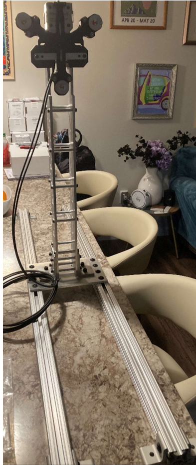
Figure 23. Assembled Series 1780 Test Stand 25 kgf 100-amp: Single Motor
