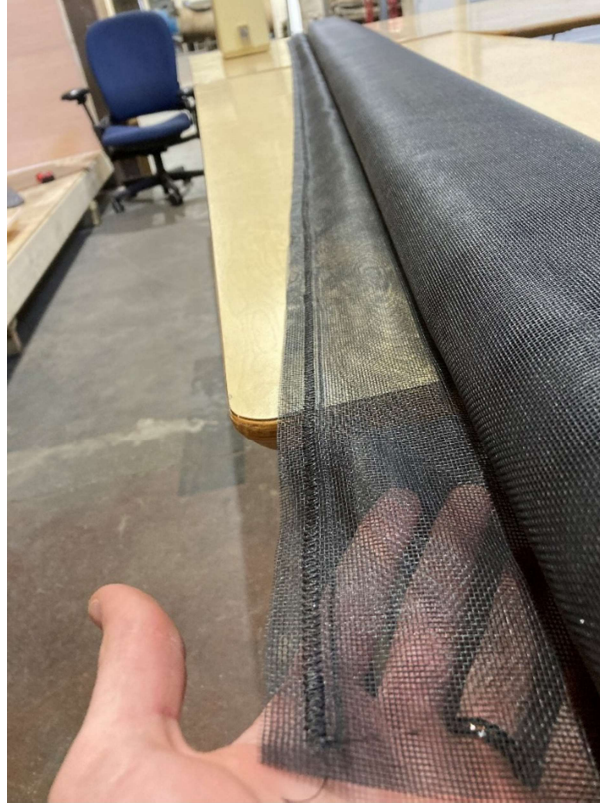
Figure 13. Fine Mesh Screen Stitching
