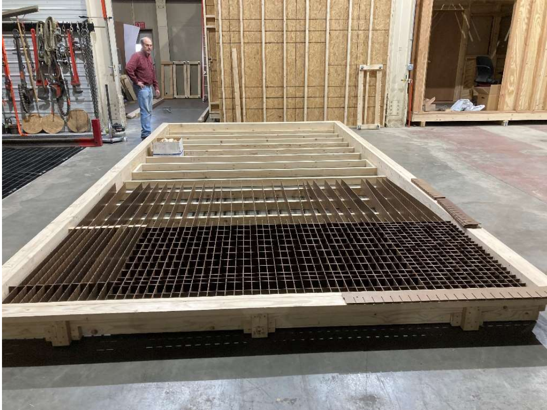
Figure 10. Flow Straightener Matrix Assembly
