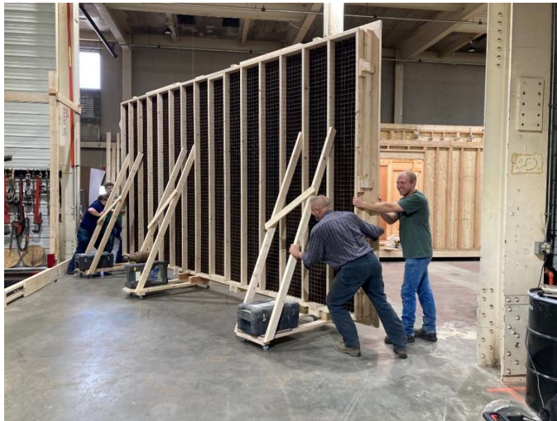
Figure 11. Mounting of Flow Straightener
