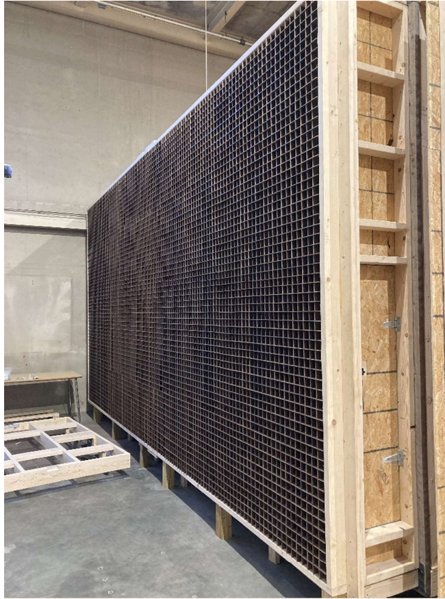
Figure 12. Completed Flow Straightener
