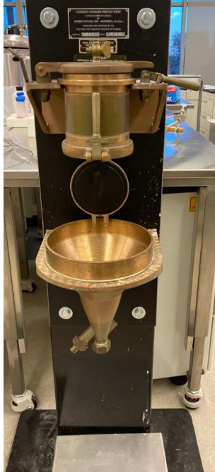
Figure 3-2 Image of the Canadian Standard Freeness Tester
