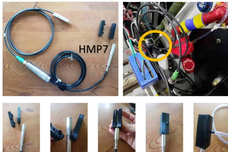
Figure 6.6: Suit gas outlet temperature and humidity are collected using a Vaisala HMP7 temperature and humidity probe located downstream of the exhaust gas of the MK III suit.
