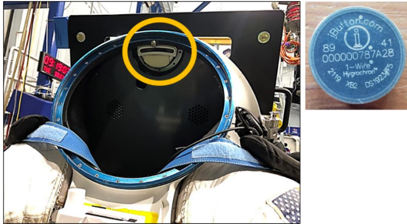
Figure 6.5: Suit gas inlet temperature and humidity collected via an iButton Hygrochron positioned at the inlet of the helmet of the MK III.
