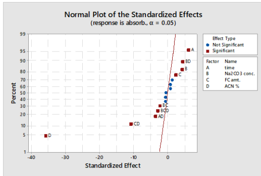
Figure 31. The normal plot of the standardized effects for 2 4 full factorial evaluation of FC phenol reactions, with four replicates (alpha = 0.05).
