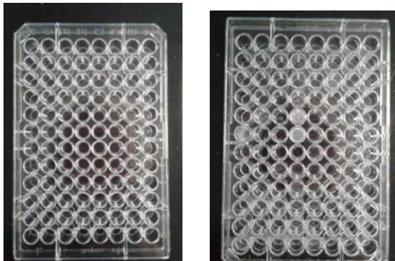
Figure 25. Left: A solution of gallic acid (100 \mu\text{g}/\text{mL} ) reacted with 50 \mu\text{L} FC reagent and 0.4 M \text{Na}_2\text{CO}_3 after two hours, with the liquid solution poured off after the reaction. Right: The same reaction after three hours (note opaque wells near the center).
