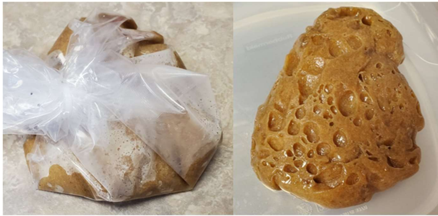
Figure 17. Fecal simulant in PDMS bag after running (Left) and once removed from the bag post processing (Right).
