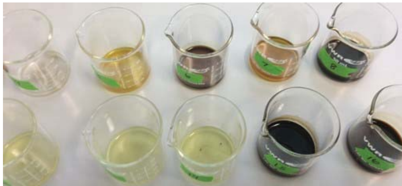
Figure 12: Extractions from Soil Samples for PFAS Identification
