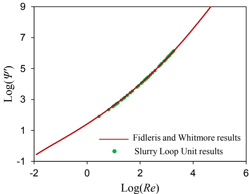
Figure B.1 – Comparison of experimental results from the Slurry Loop Unit experimental work and the work of (Fidleris and Whitmore, 1961a, 1961b).
