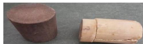
Figure 3.20: Lateral and longitudinal breaking for the 3D printed core sample to check the effect of CO<sub>2</sub>
