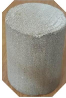
Figure 4.2: Original Berea sandstone core plug (1.5 inches in diameter and 2 inches in length)
