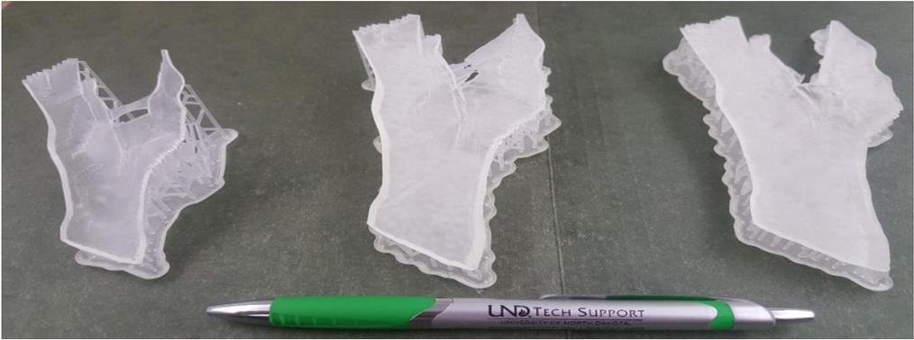
Figure 5.13: 3D-Printing the meshed geometry of E-Segment of Norne field in the North Sea in three different sizes [166]
