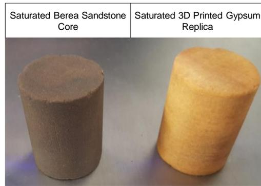
Figure 4.25: Saturated Berea core sample and its gypsum replica with Bakken oil
