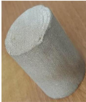
Figure 1.1: Original Berea sandstone core plug (1.5 inch in diameter and 2 inch in length)
