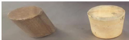
Figure 3.19: Samples after CO<sub>2</sub> injection at 3500 psi
