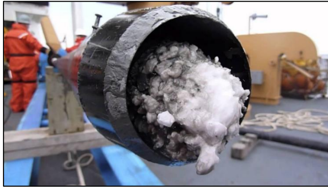
Figure 2.10 Gas hydrate plugging of gas transportation pipeline (Polartrec.com)
