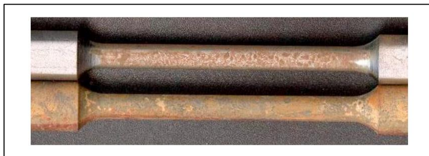
Figure 2.11 General view of corrosion damage of the specimen after exposure to gas hydrates (Poberezhny, et al 2019).
