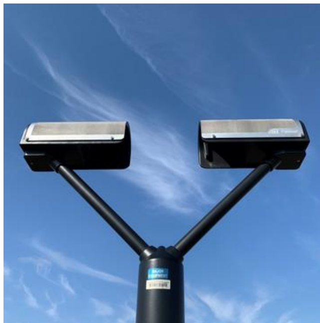
Figure 9. Image of a Parisvel 2 optical disdrometer at the University of North Dakota Oakville Prairie Observatory taken by Aaron Kennedy.
