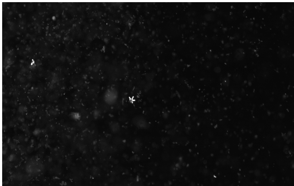
Figure 3. Image from Dr. Aaron Kennedy's snowflake camera in Grand Forks, North Dakota at 07:31:13 UTC on 12 February 2020 showing several broken snow crystals (appearing as brighter particles) surrounded by other fragmented (darker) BLSN particles.
