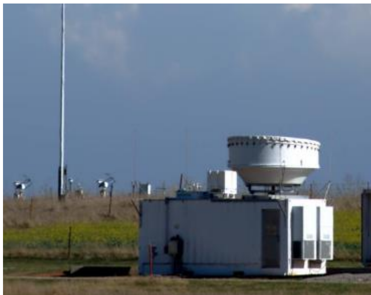
Figure 16. Image of the KAZR deployed at DOE ARM Southern Great Plains site (Widener et al. 2012).
