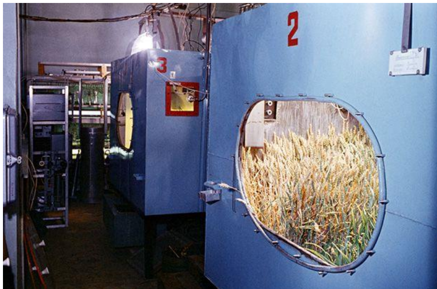
Figure 23 Bios-2 Algal Cultivator and Phytotron (Sohail, 2015)
