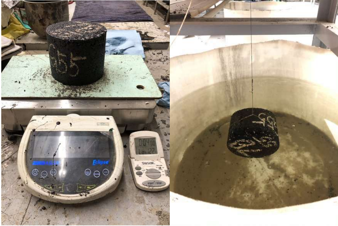
Figure 20. Sample Asphalt plug weighed in air and Sample submerged under water
