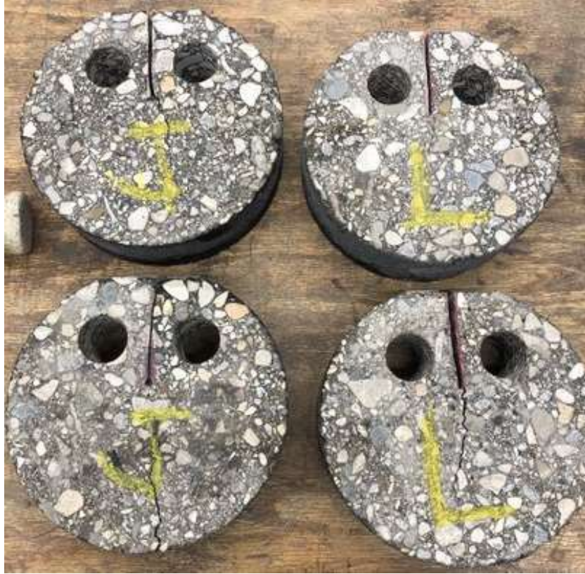
Figure 37. Typical sample after DCT test
