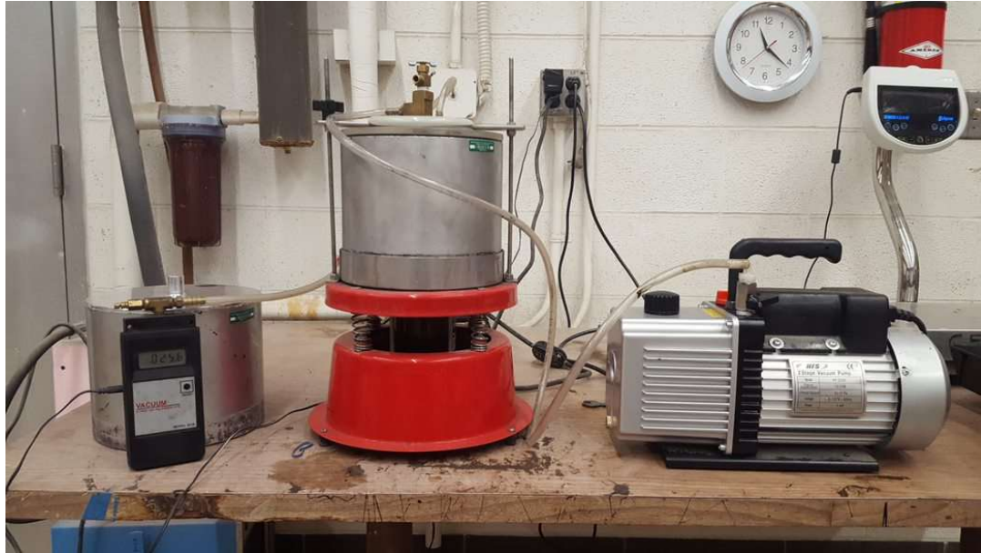
Figure 17. Theoretical Maximum Specific Gravity ( G_{mm} ) Experiment Set-up
