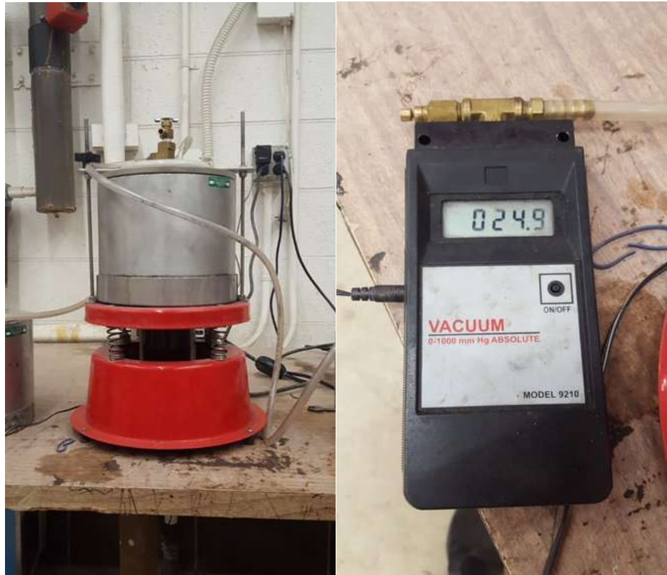
Figure 16. Set-up of bowl and Vacuum Gauge
