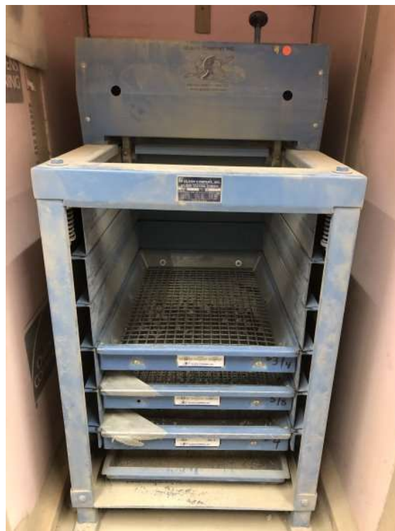
Figure 14. Common set-up of Mechanical Shaker
