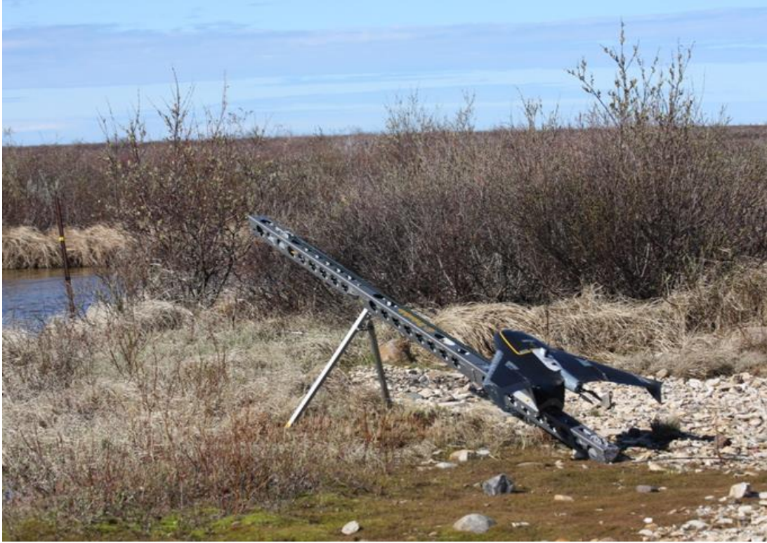
Appendix A Figure 1 The Trimble UX5 on the elastic catapult launcher. Photo credit Dr. Susan Ellis-Felege (June 2015).
