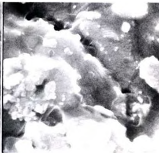
FIGURE 14. - Nahcolite treated at 900 °F - final stage of sintering. (Two hour treatment.)
