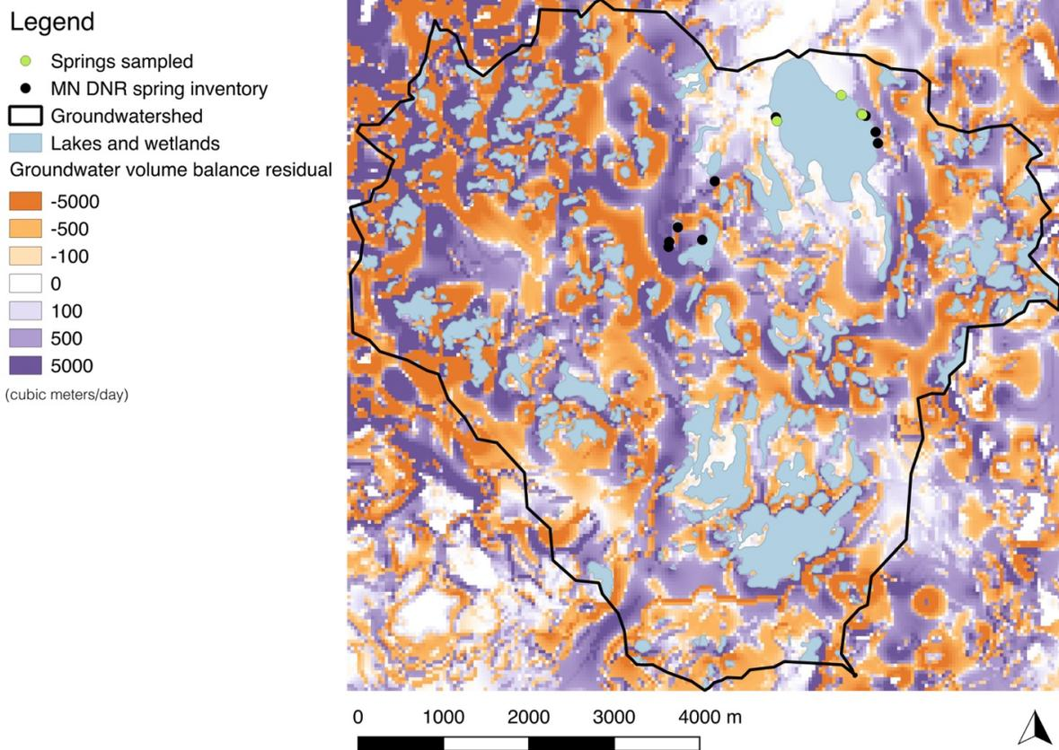
Figure 21. Recharge-discharge map for the study area computed from the unfilled 40-meter interpolated water-table surface.
