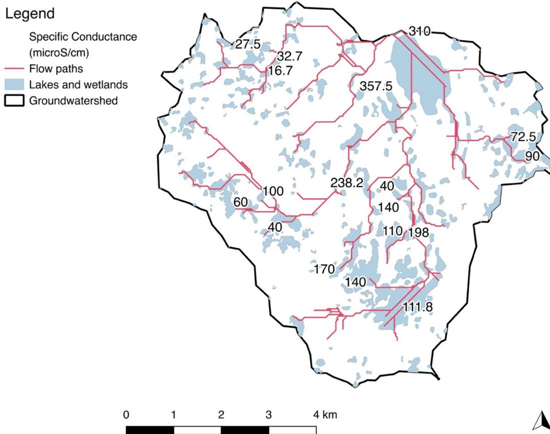
Figure 15. Groundwater flow path lines (in red) for the study area with specific conductance measurements for sampled lakes and wetlands.
