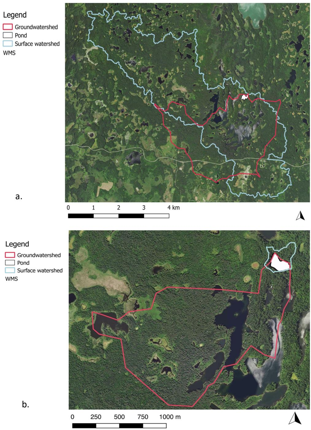
Figure 18. a. Surface watershed and groundwater watershed delineated for a sampled pond. This pond had a watershed area ratio of 2.17. b. Surface watershed and groundwater watershed delineated for a sampled pond. This pond had a watershed area ratio of 0.04.
