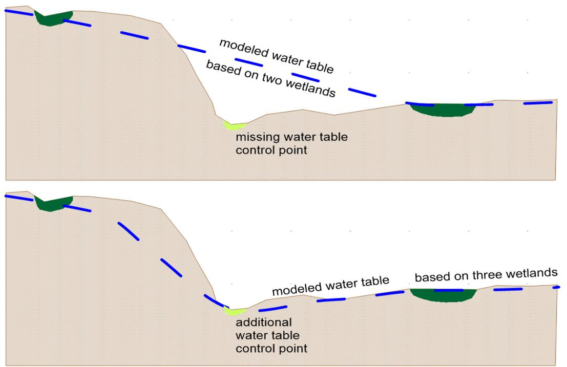
Figure 5. Profile diagram showing the effect of adding additional water-table control in an area of complex topography.
