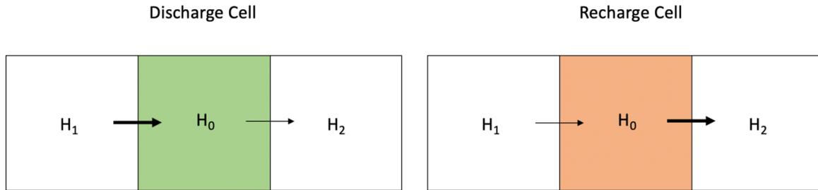
Figure 7: Example of groundwater recharge and discharge cells in the volume balance residual raster. The bold arrow represents a higher magnitude of flow.
