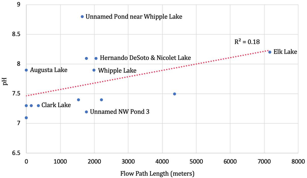
Figure 14. Graph of flow path lengths and pH measurements for sampled lakes and wetlands.
