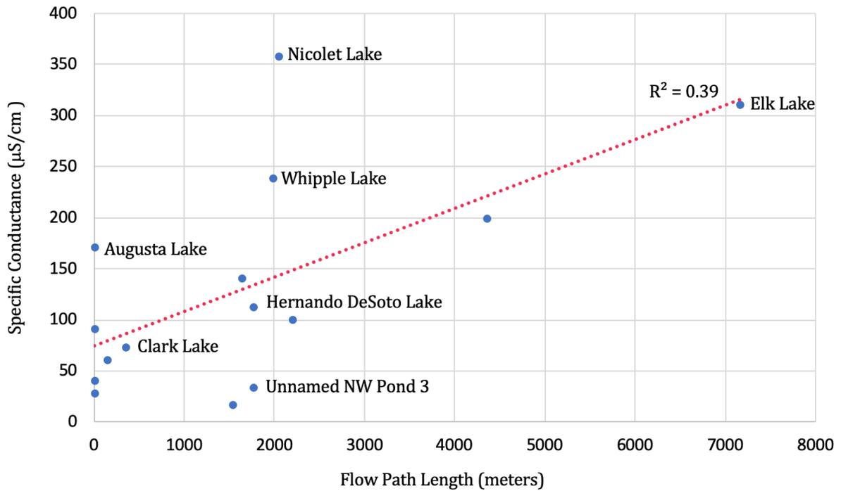
Figure 16. Graph of flow path lengths and specific conductance measurements for sampled lakes and wetlands.
