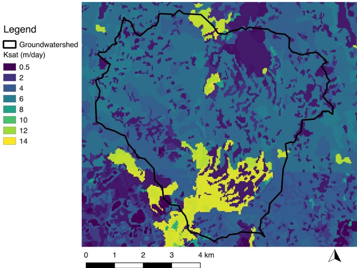
Figure 8.  $K_{sat}$  values for the study area from the SSURGO soil polygons (Soil Survey Staff 2019; Wiczorek 2014).
