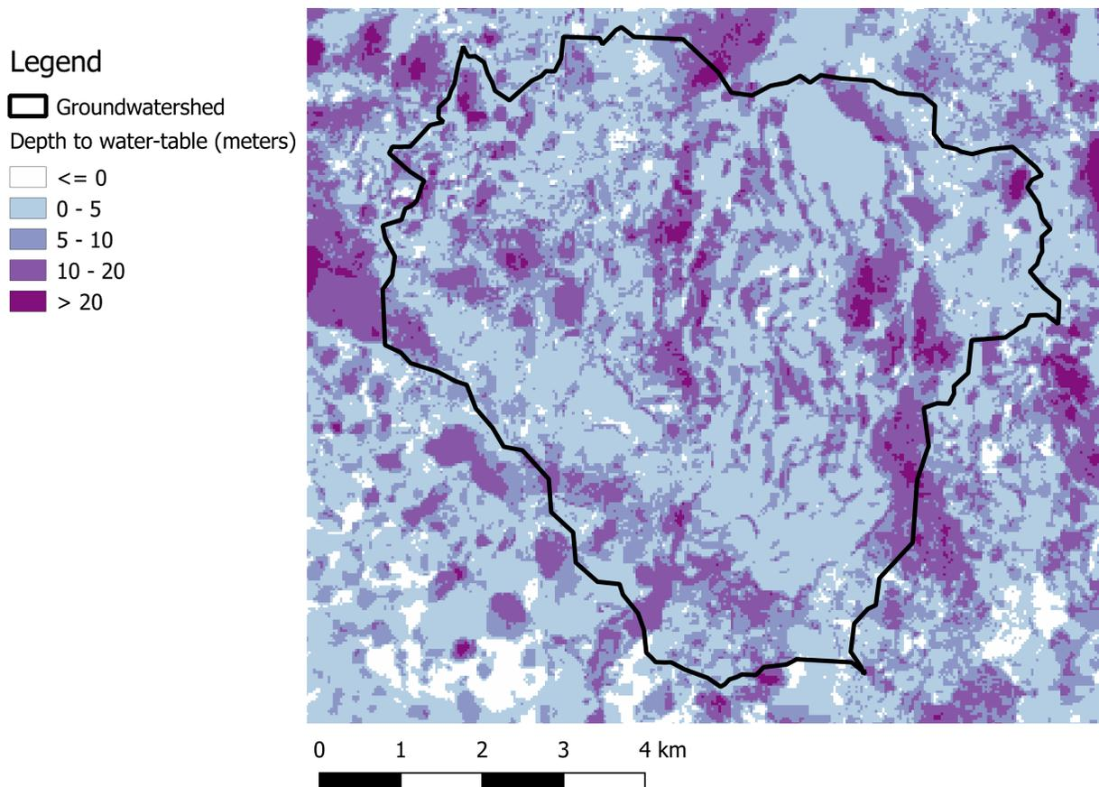
Figure 11. The depth to the interpolated water-table surface for the study area. Shown in white are areas where the interpolated water-table surface lies above the DEM.
