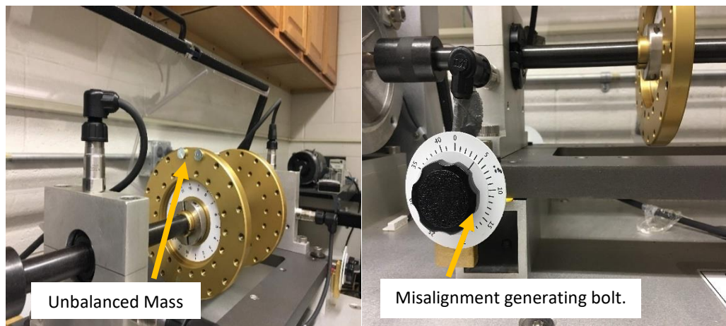
Figure 2. 4 Unbalanced and misaligned condition simulation.
