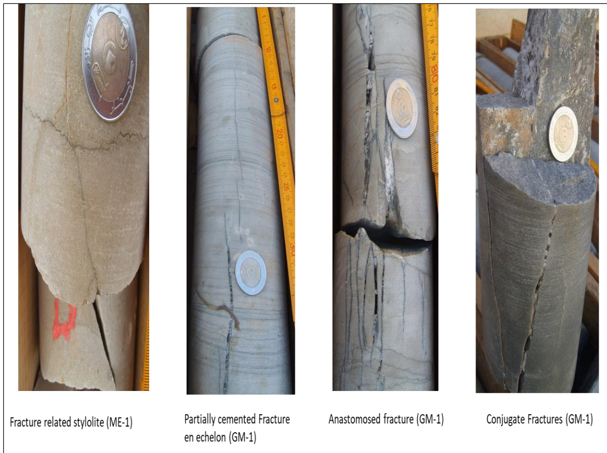
Figure 54: Example of Mode IV and Mode I fractures that affect the Ordovician reservoir.
