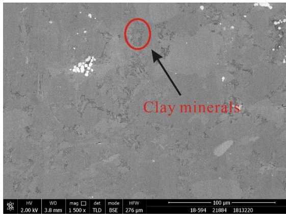
(a) Clay minerals in the intergranular pores of calcareous siltstone, low organic content
