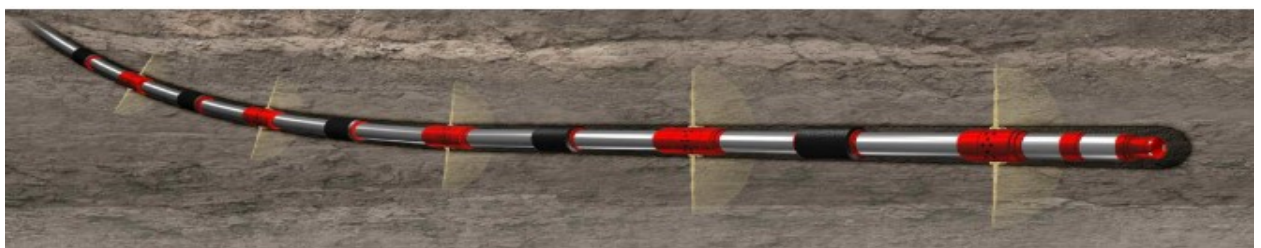
Figure 7. Multi-stage hydraulic fracturing (Rafie et al., 2014)
