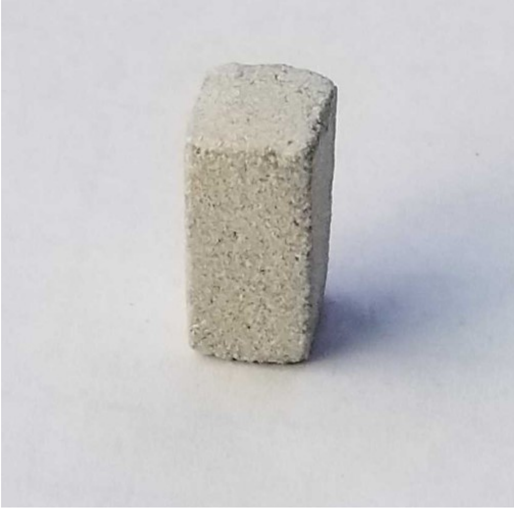
Figure 11. Core sample prepared for CT scan
