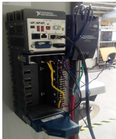
Figure 4.5 The Data logging system used for the blockage experiments
