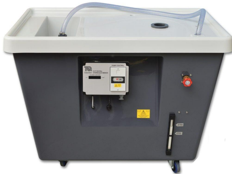
Figure 4.2 The H1D volumetric hydraulic bench
