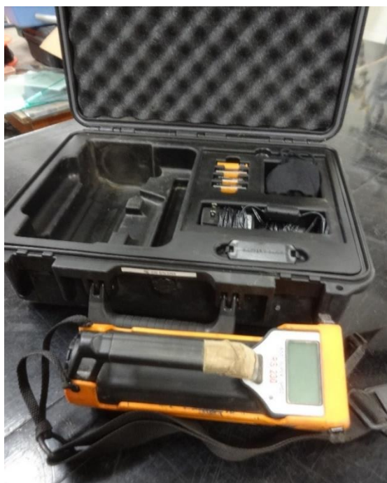
Figure 14. HHSgge Geothermal Laboratory's RS-230 BGO GRS portable radiation detector
