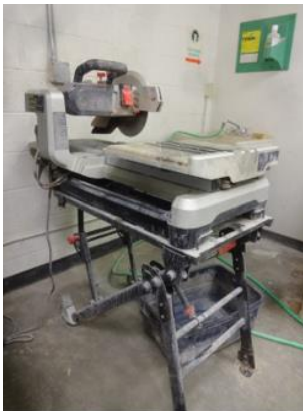
Figure 8. Rock saw in the sample preparation room used to cut large rocks into smaller segments that would fit inside of the rock crusher. The saw assisted in separating and removing the weathered sections of the samples.
