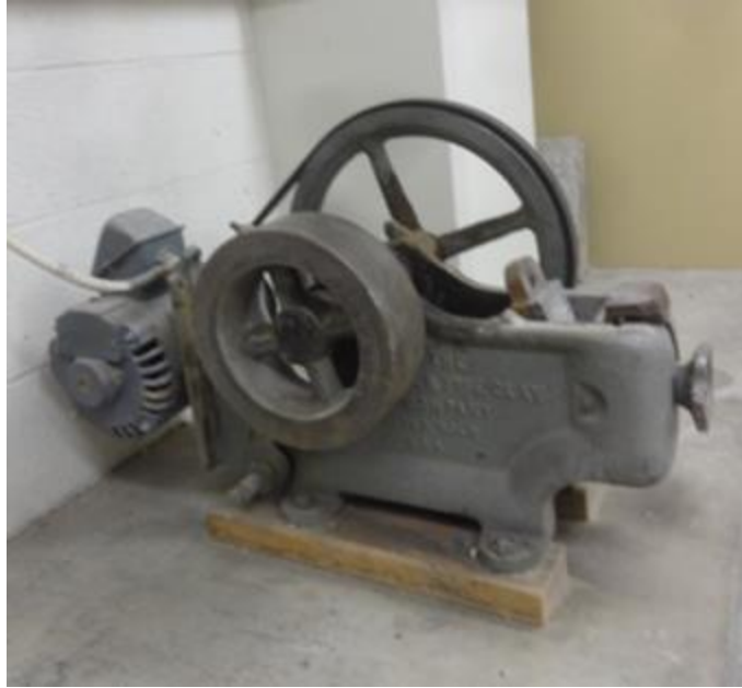
Figure 10. Rock crusher used to crush the fresh, clean section of rocks into 2-cm by 2-cm fragments. The paper storage container (Fig. 11) would be placed under the open section of the crusher to catch the small fragments.
