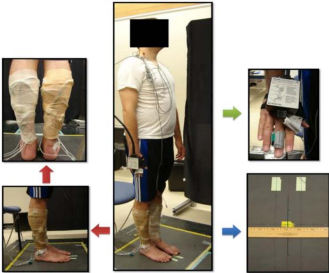
Figure 4.2. An example of experimental setup for acquisition of simultaneous blood pressure, calf electromyography, and postural sway (Centre). Calf electromyography acquired from four different leg muscles (left). Force platform right (bottom), and finger plethysmography (top right)(146).
