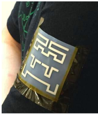
Fig. 2.5: Flexible antenna mounted on the human chest [43].
