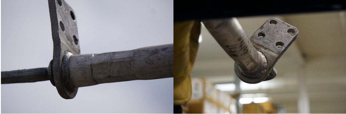
Figure 26: Example images in which the DEBC weld detector failed to detect the weld.
