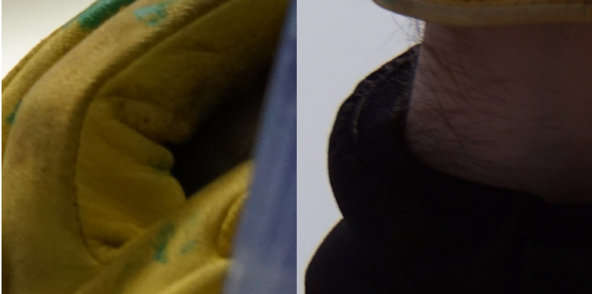
Figure 27: Example images of false positive DEBC weld detections cause by a glove to the left and the sleeve of a jacket to the right.
