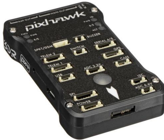
Figure 34:Image of the PIXHAWK Autopilot
