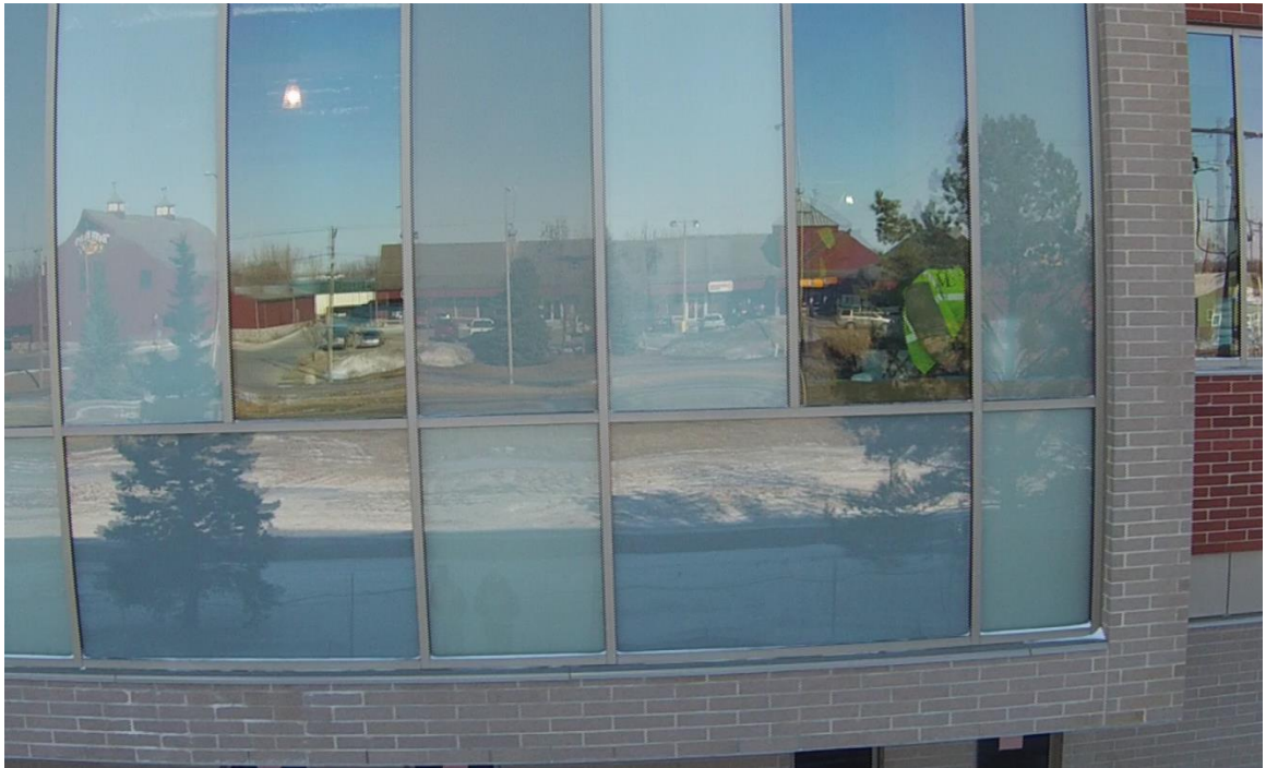
Figure 39: Example of an environment with reflective surfaces. The algorithm fails to detect and track sufficient distinctive corner points for accurate camera pose estimation.
