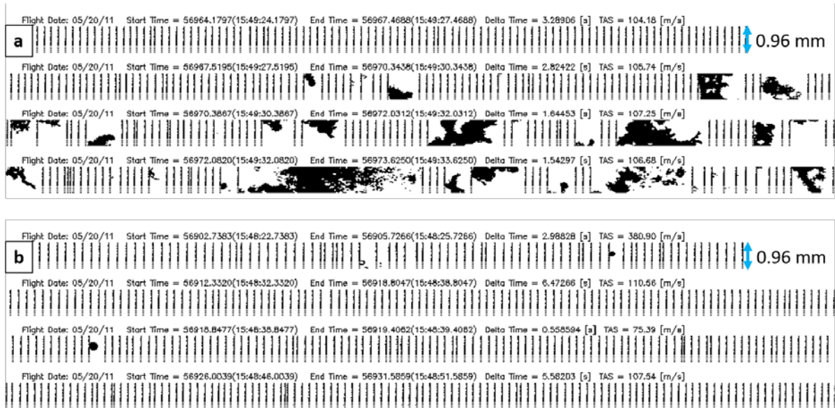
Figure 5-13: Particle images from the 2DC from the 20 May 2011 flight between a) 15:49:24.2 and 15:49:33.6, b) 15:48:22.7 and 15:48:51.6 UTC. Horizontal lines denote the start/end point of images. Image array width (blue arrow) is 0.96 mm.
