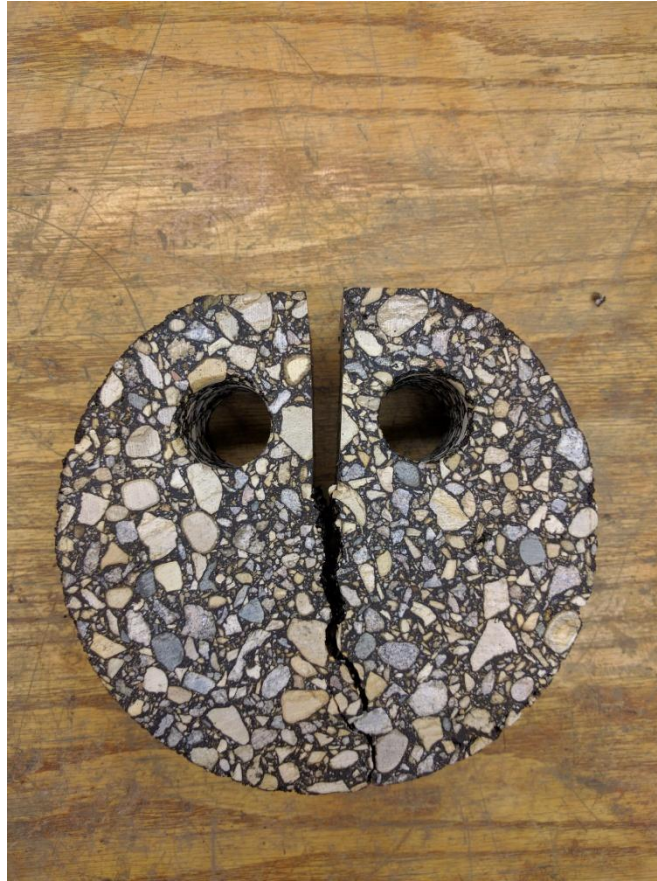
Figure 20. Sample DCT Test Specimen
