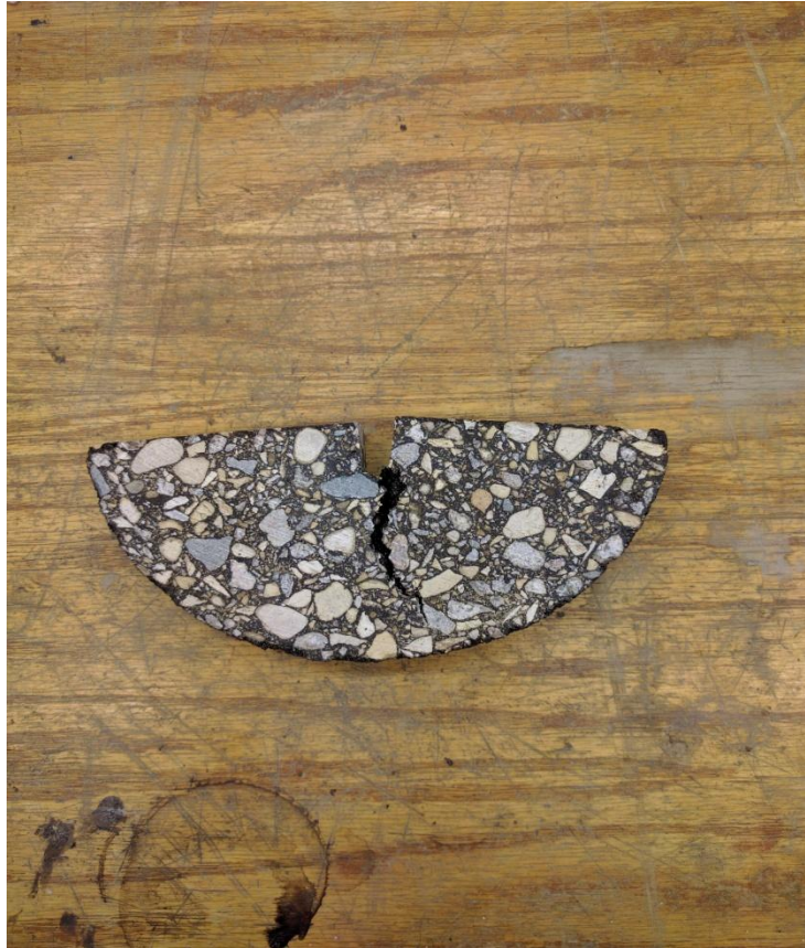
Figure 24. Sample SCB Test Specimen
