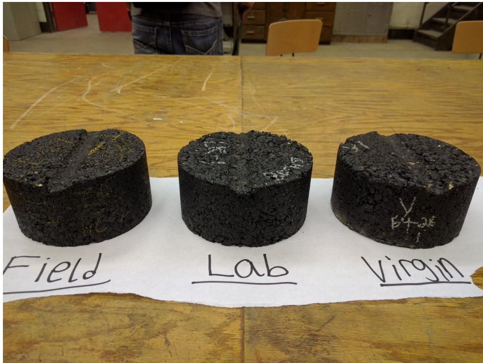
Figure 11. PG64-28 Sample Rutting Specimens
