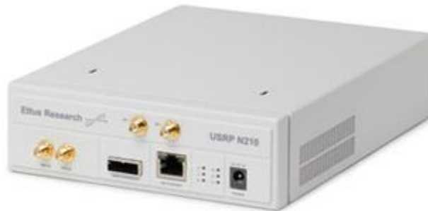
Figure 43. Universal Software Radio Peripheral Software Defined Radio from Ettus Research
