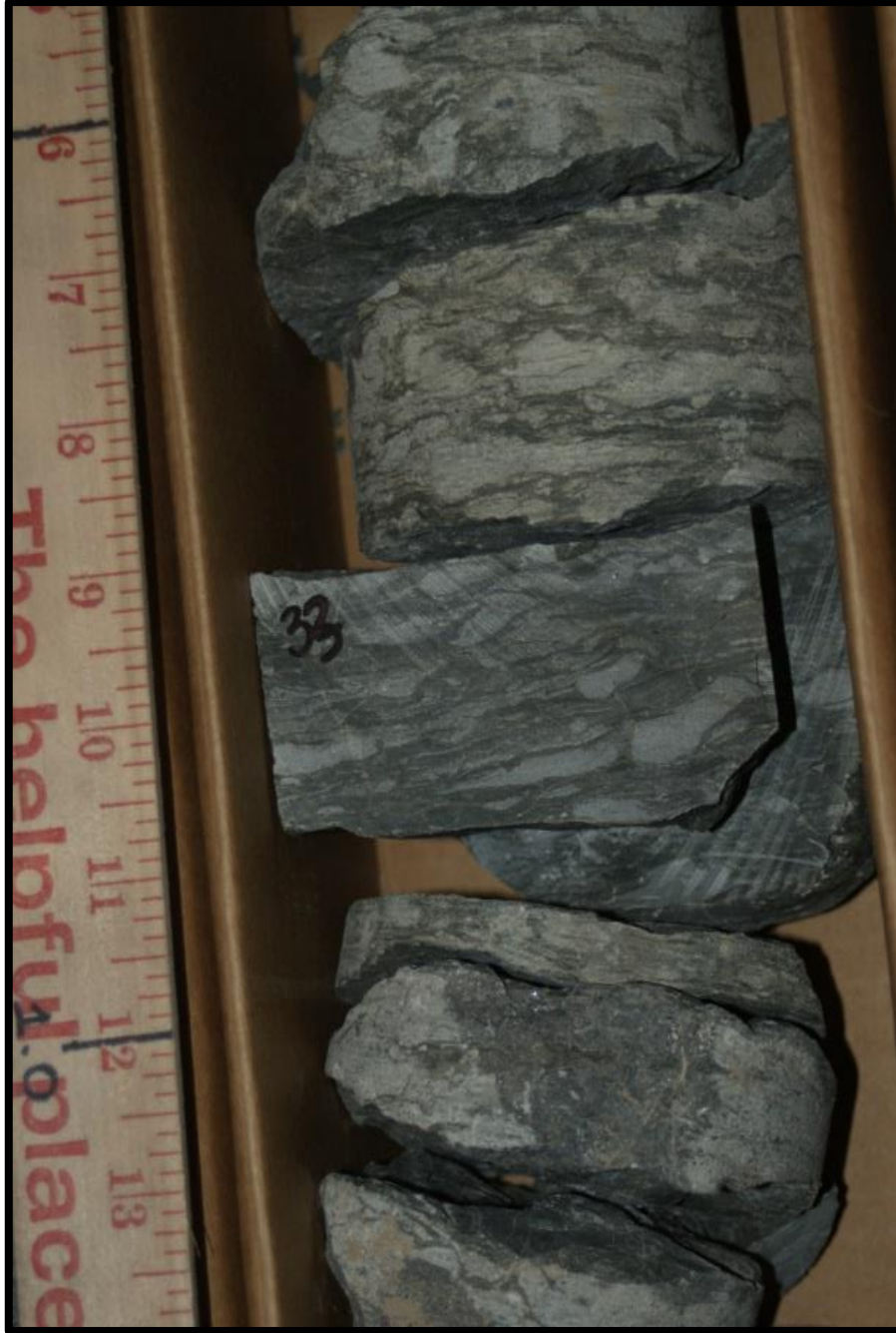
Figure 18. A photograph of core from NDGS #291 at a depth of 13,233'. An example of the burrow-mottled, silty, calcareous mudstone at the base of Member D. The ruler is in inches.
