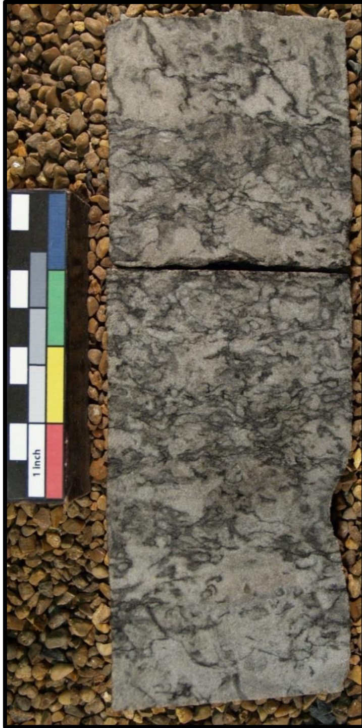
Figure 25. A photograph of core from NDGS #13405 at a depth of 14,330'. Displaying intense horizontal and vertical burrows.
