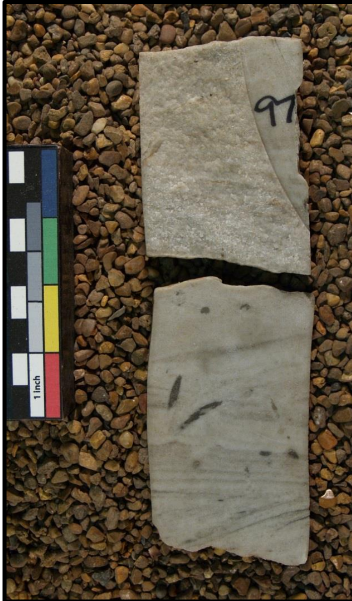
Figure 22. A photograph of core from NDGS #3268 at a depth of 12,797'. Cross-bedded quartz arenite which occurs at the base of Member E.
