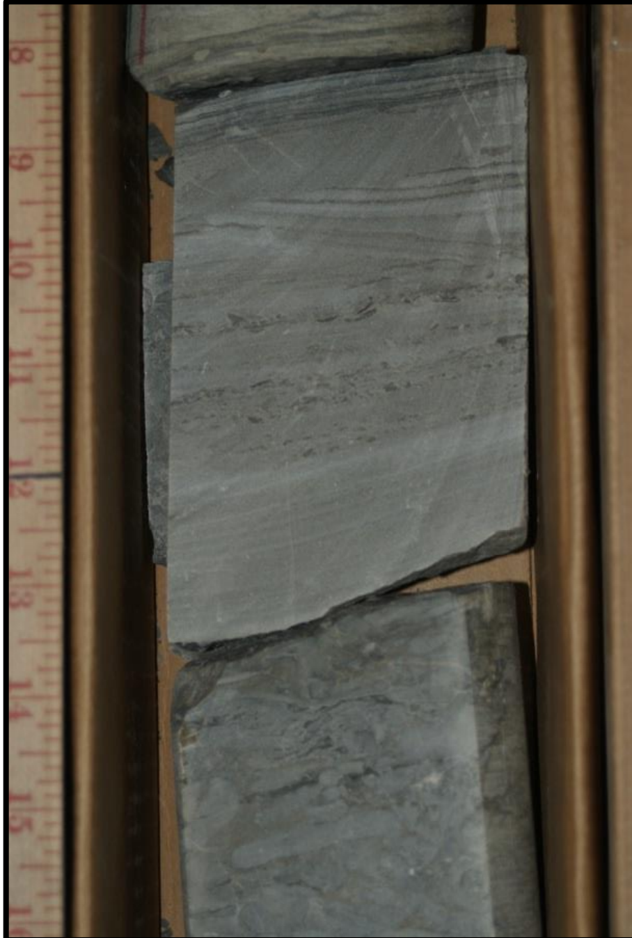
Figure 20. A photograph of core from NDGS #291 at a depth of 13,171'. An example of the siltstone and sandstone overlying the mudstone. The ruler is in inches.
