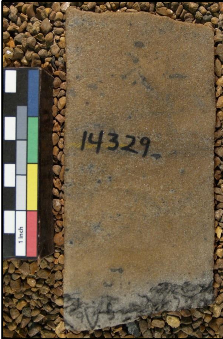
Figure 24. A photograph of core from NDGS #13405 at a depth of 14,329. Displaying hydrogen sulfide staining.
