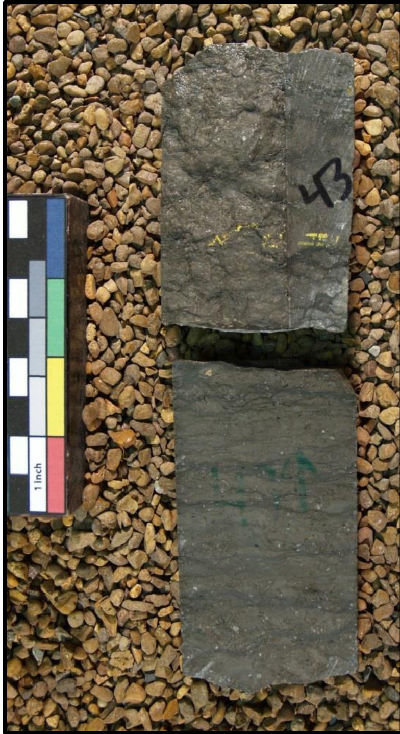
Figure 23. A photograph of core from NDGS #3268 at a depth of 12,643'. An example of the fossiliferous limestone lithotype which occurs at the top of Member E.
