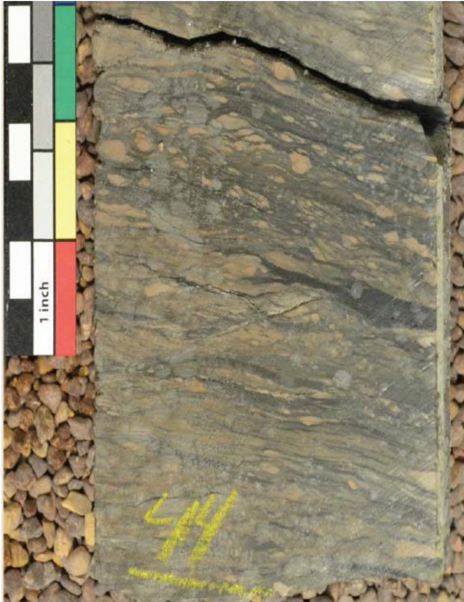
Figure 20. Mottled Beds. Mottled bed unit from the North Plains Energy, LLC Sorenson 160-100-27--34-4a (48.661817 N 103.596372 W) at 9144 ft (photo courtesy of the NDIC)
