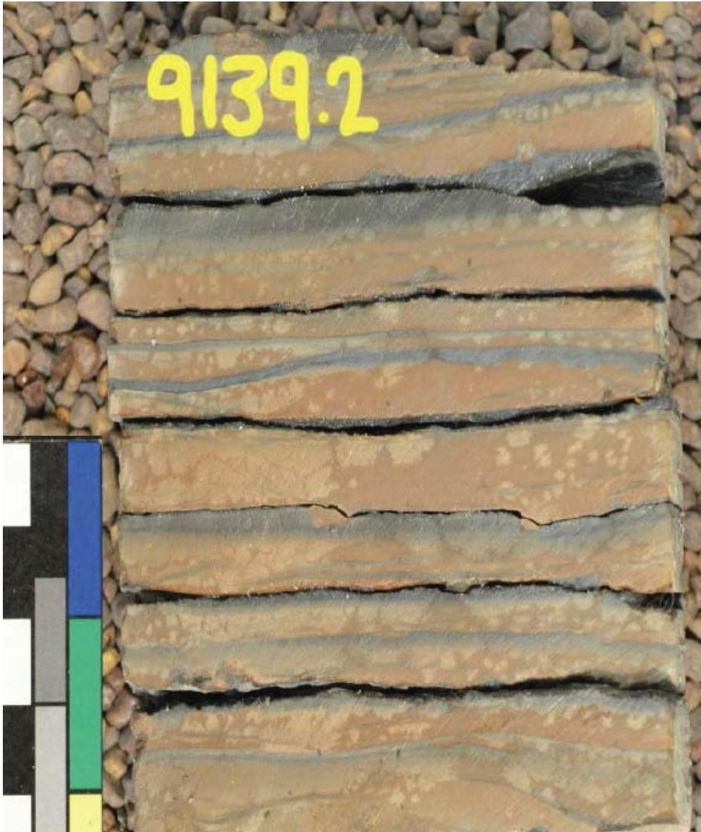
Figure 6. Laminated Beds. Laminated bed unit from the North Plains Energy, LLC Sorenson 160-100-27--34-4a (48.661817 N 103.596372 W) at 9139 ft (photo courtesy of the NDIC).
