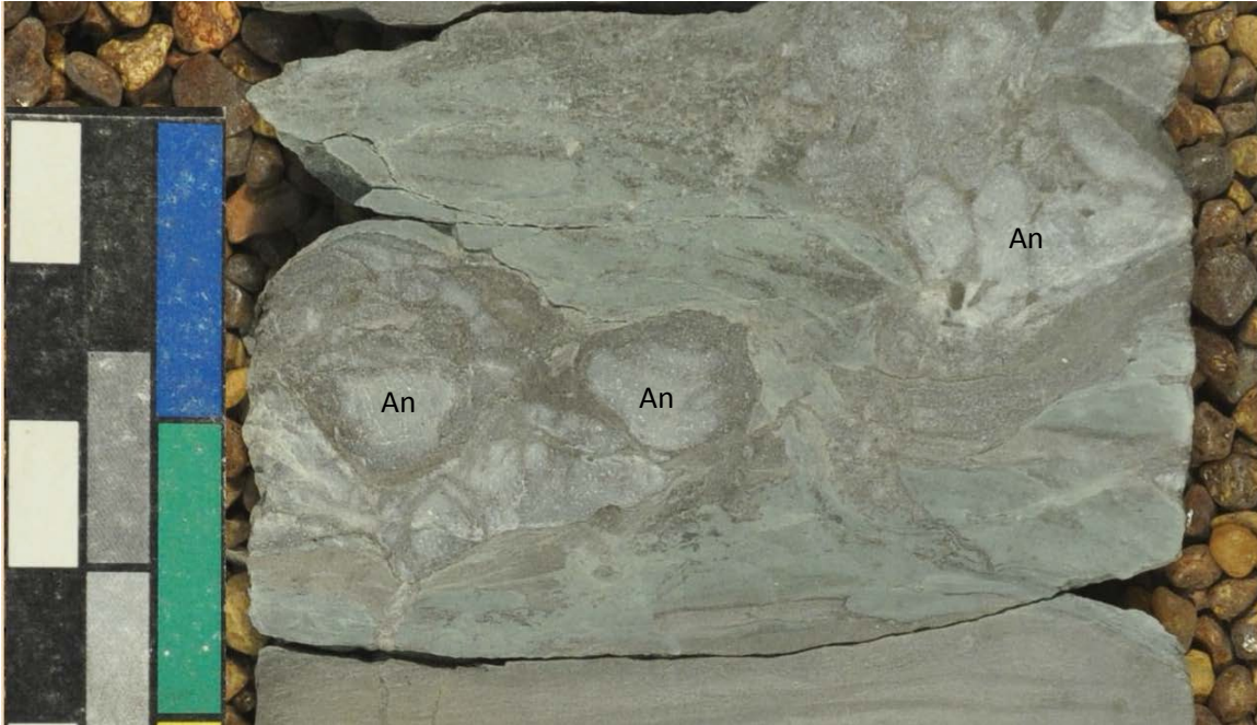
Figure 23. Anhydrite Nodules in Member 6. Anhydrite nodules from Continental Resources, INC. Charlette 1-22H (47.964578 N 103.333939 W at 11356 ft (photo courtesy of the NDIC)
