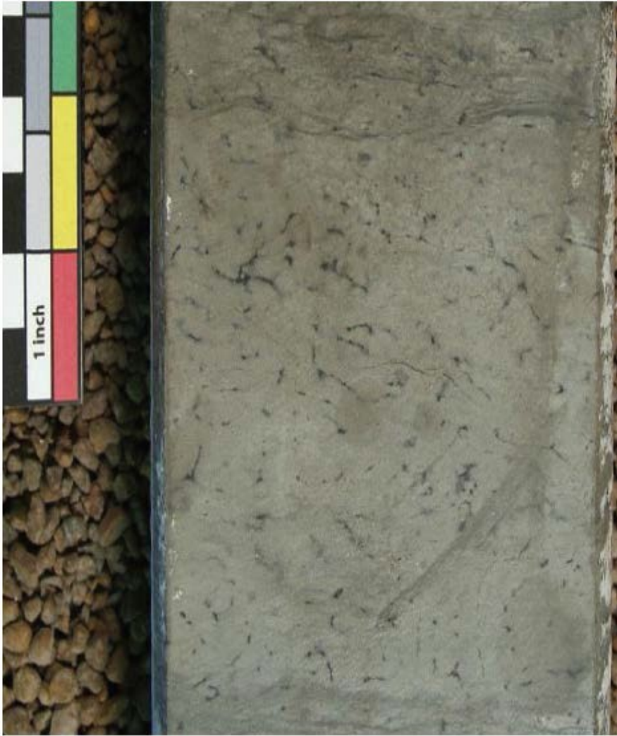
Figure 26. Pattern Dolomite. Pattern dolomite from the SM Energy Company Willard Johnson Trust 24B-2-1H (48.674960 N 103.426239 W at 9218 ft (photo courtesy of the NDIC)
