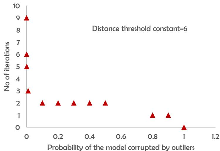
**Figure 4.5: Performance vs computation of the RANSAC algorithm at a constant distance threshold value for an example image pair.**
