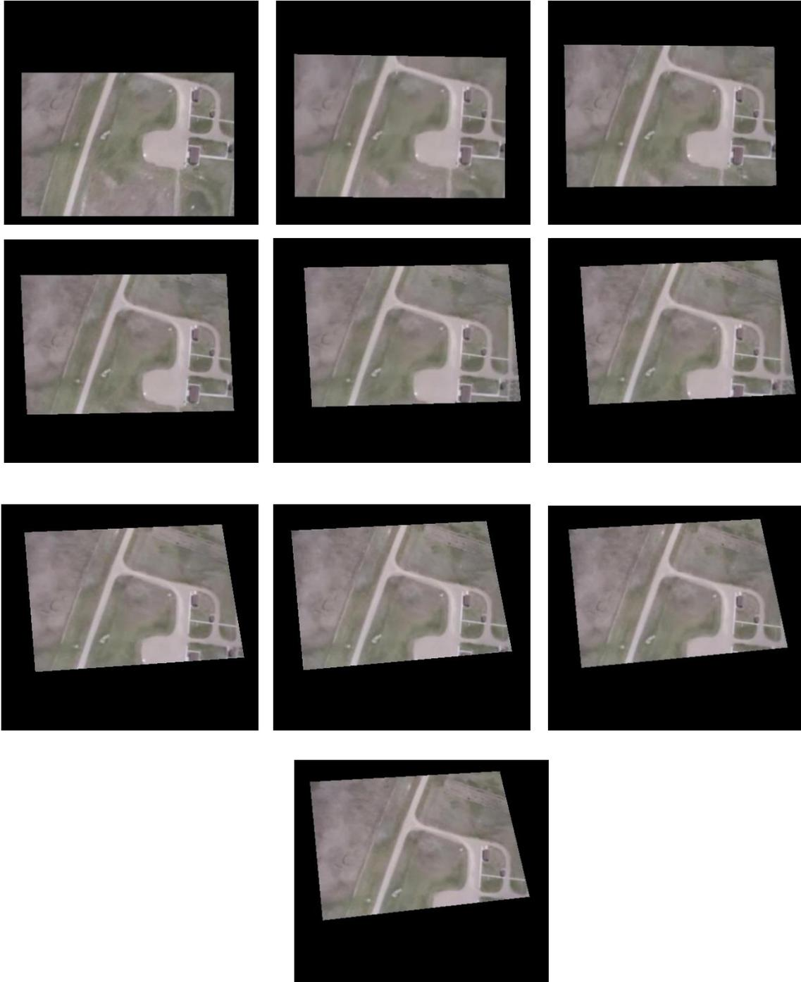
Figure 4.10: Projection of frames into common coordinate.
