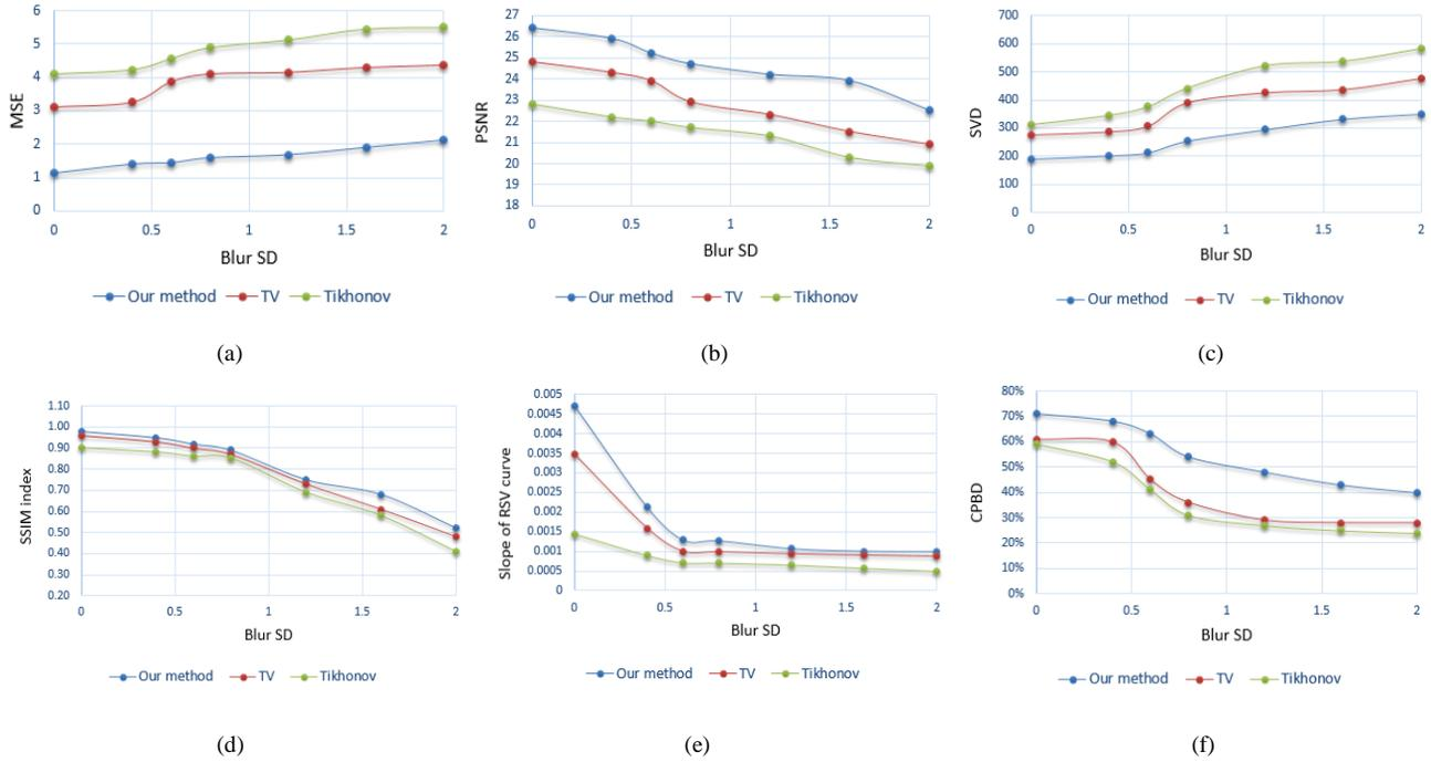
**Figure 5.9: Behavior of performance metrics in the presence of blur. (a) MSE behavior; (b) PSNR behavior; (c) SVD behavior; (d) SSIM behavior; (e) behavior of RSV curve's slope; (f) CPBD behavior for a single dataset.**
