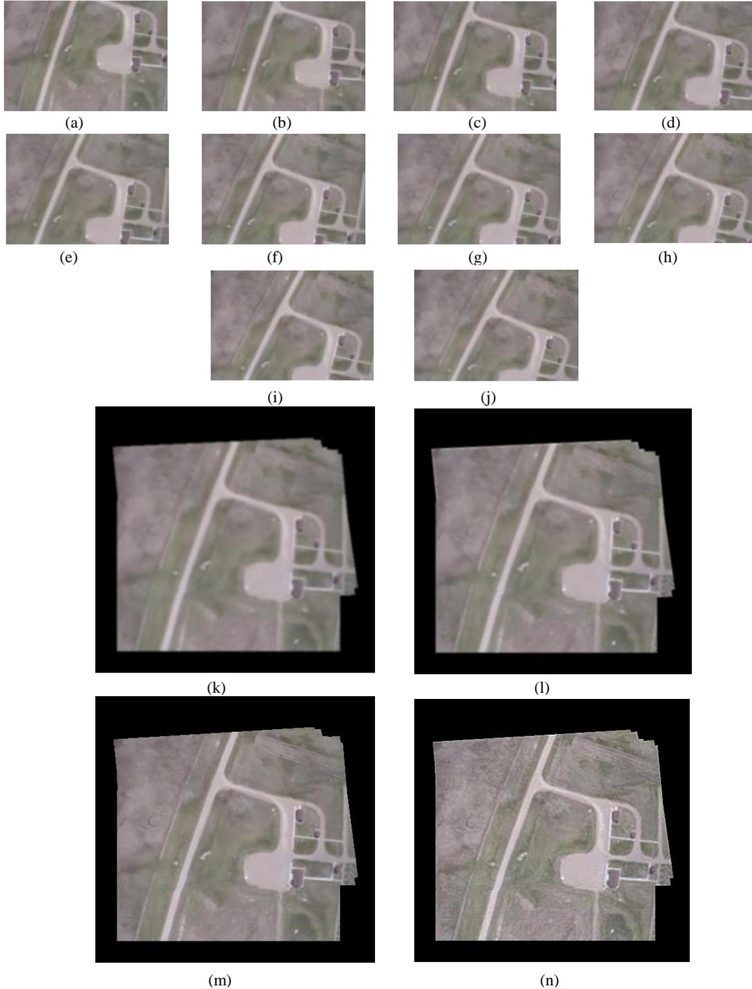
**Figure 5.5: SR result using simulated UAV data. (a)-(j) LR input frames; (k) Mosaic without SR; (l) Mosaic with Tikhonov regularization-based SR; (m) Mosaic with TV regularization-based SR; (n) Mosaic with proposed algorithm.**
