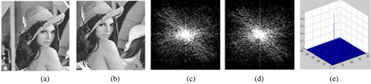
**Figure 2.6: Use of cross-power spectrum to detect transformation. (a), (b) Source images with displacement between them; (c), (d) Corresponding spectrum; (e) Impulse function indicating displacement between the images.**
