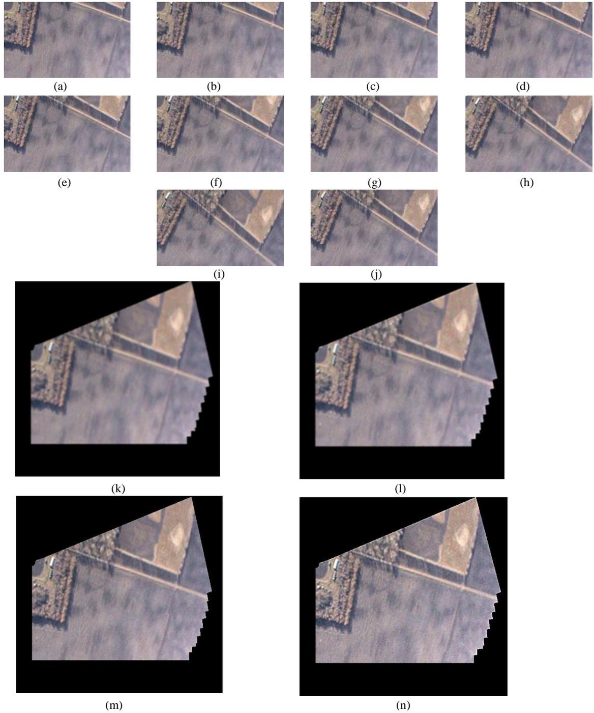
**Figure 5.3: SR result using simulated balloon data. (a)-(j) LR input frames; (k) Mosaic without SR; (l) Mosaic with Tikhonov regularization-based SR; (m) Mosaic with TV regularization-based SR; (n) Mosaic with proposed algorithm**
