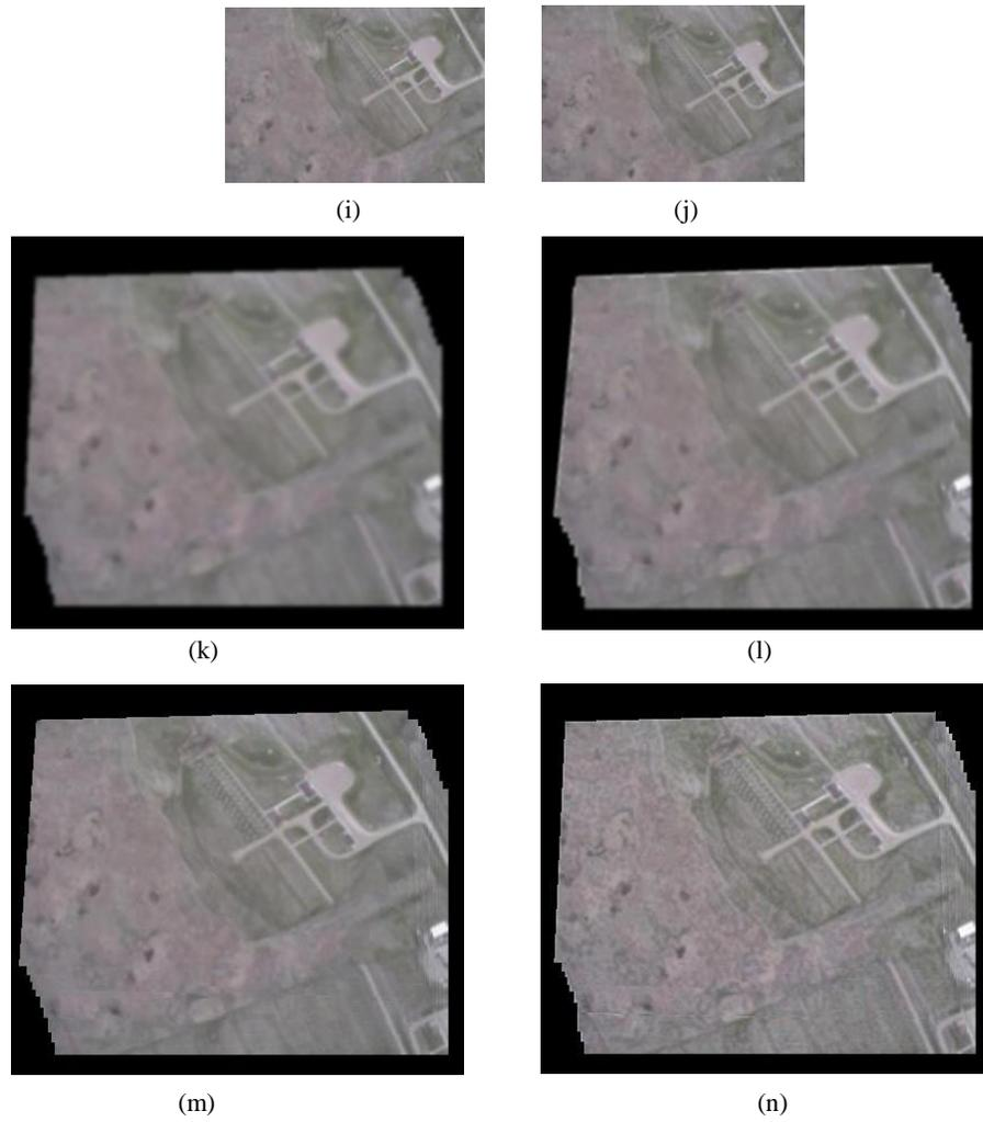
**Figure 5.7: SR result using real UAV data. (a)-(j) LR input frames; (k) Mosaic without SR; (l) Mosaic with Tikhonov regularization-based SR; (m) Mosaic with TV regularization-based SR; (n) Mosaic with proposed algorithm.**
