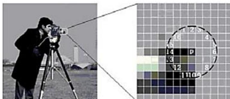
**Figure 2.3: Candidate feature detection for FAST algorithm.**
