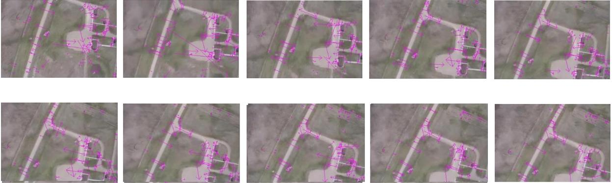
**Figure 4.8: SIFT features extracted from the input frames.**
