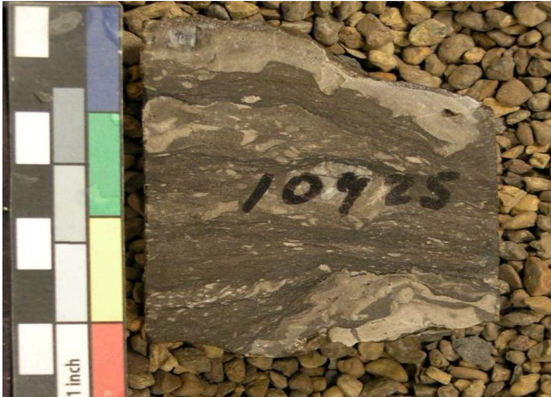
Figure 19. NDGS 859. 10925 ft. Anhydrite limestone.
