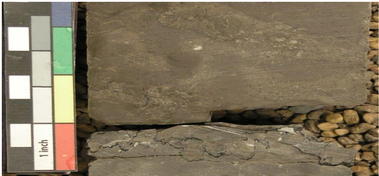
Figure 16. NDGS 291. Depth. 10691-2 ft. A packstone showing biosparite and stylolite.
