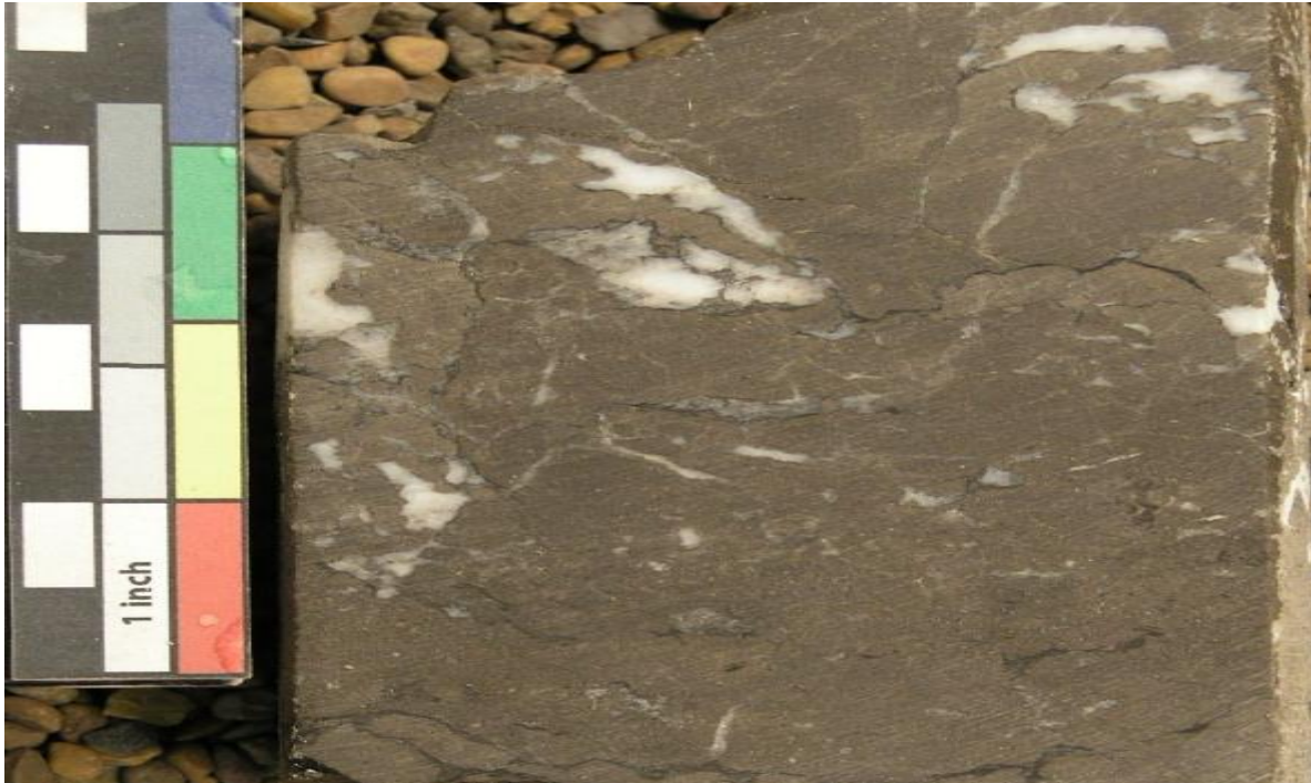
Figure 17. NDGS 291. 10681-5 ft. Patches of anhydrite limestone with fractures.
