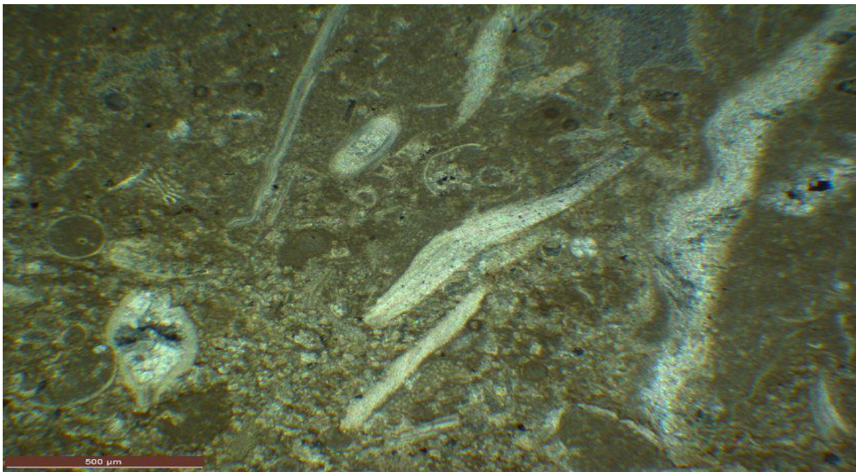
859 (10925-26 ft.) A packstone showing bivalve, echinoid and brachiopod forming a biosporite with micrite envelopes projecting the outline of the original structures.
