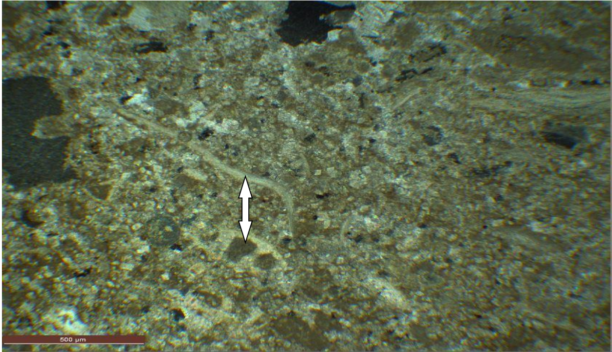
859 (10925-26 ft.) This packstone shows gastropod and brachiopod fragments embedded in a limestone with dolomite crystals
