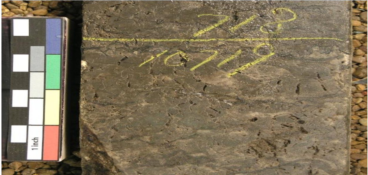
Figure 22. NDGS 15412. 10719-0 ft. Highly burrowed with stylolites.
