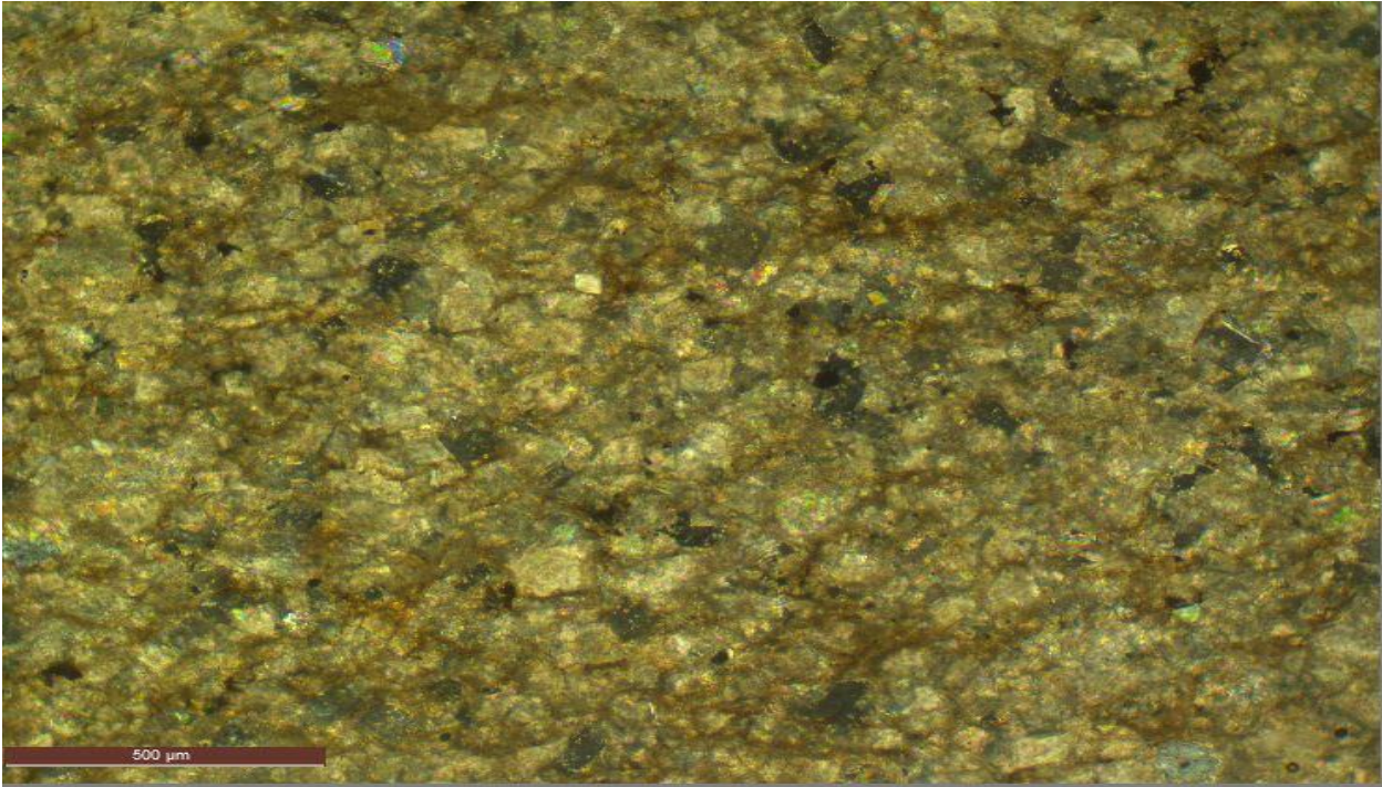
291 (10685 ft.) Packstone partially dolomitized but with lots of the “ghost” of the original sediment visible by the micrite envelopes.
