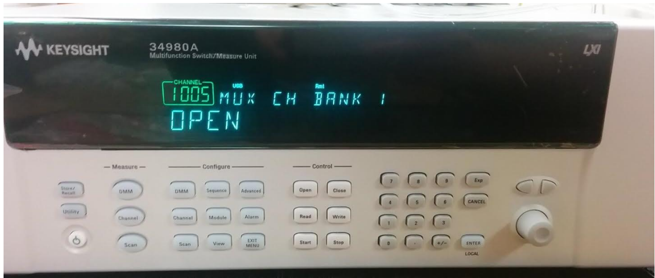
Figure 45: Keysight data acquisition system used in testing.
