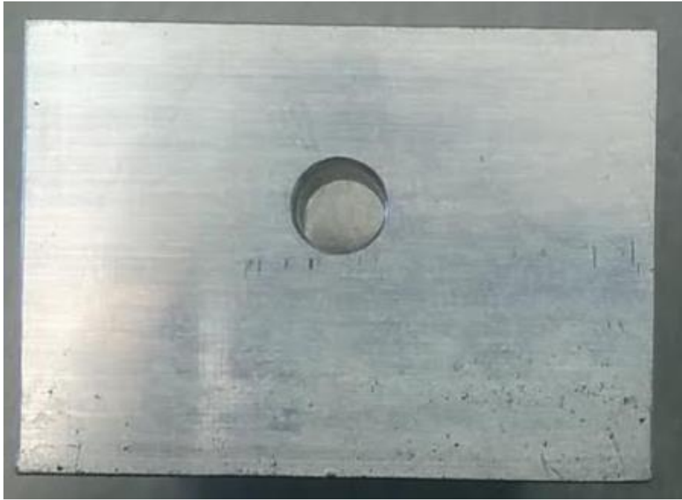
Figure 40: Inlet and outlet hole connecting the reservoir to the system tubing.
