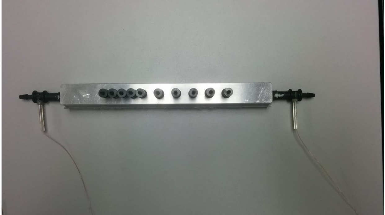
Figure 33: Image of test expansion and contraction test section. The square section is on the left side of the image and the rectangular, larger channel is on the right side.
