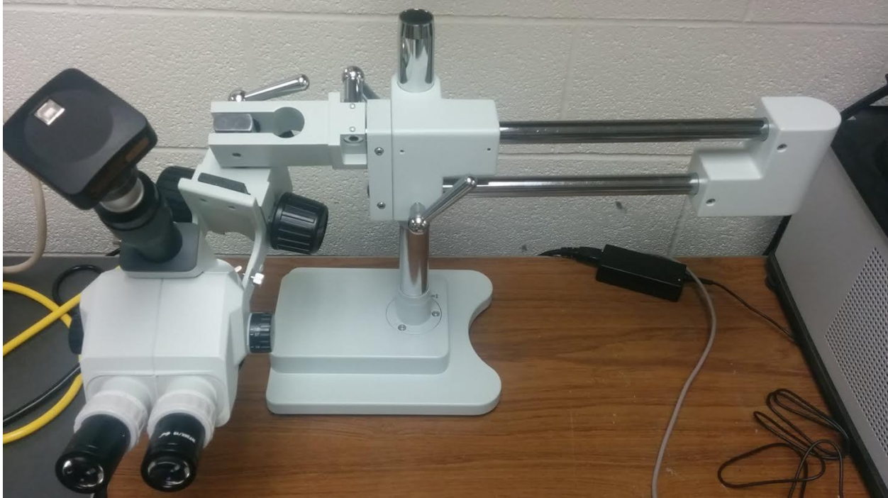
Figure 42: Amscope microscope with boom and optional digital camera.
