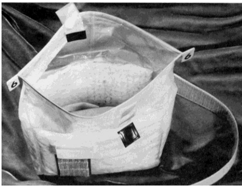
Figure 26. Protective padded sample bag (Allton, 1989) (NASA photo S72-43790).
