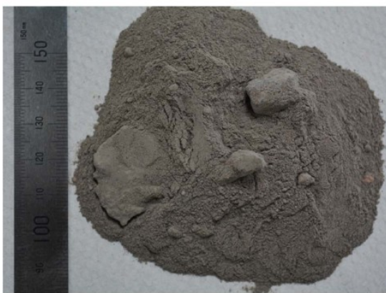
Figure 33. BP-1 Lunar Regolith Simulant (Suescun-Florez et al., 2015).
