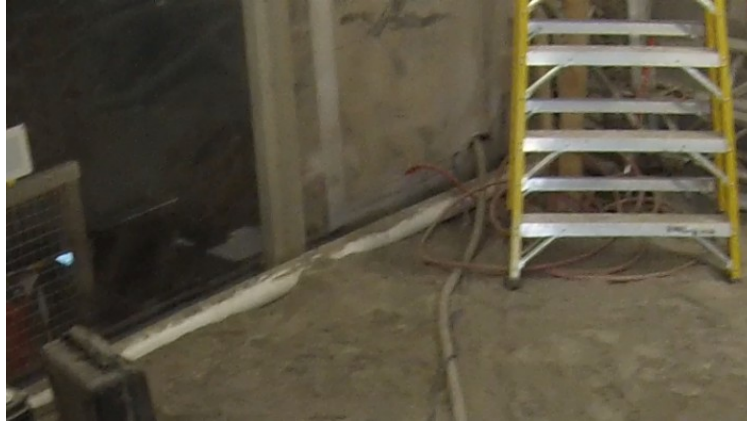
Figure 56. Air umbilical being fed into the regolith bin.
