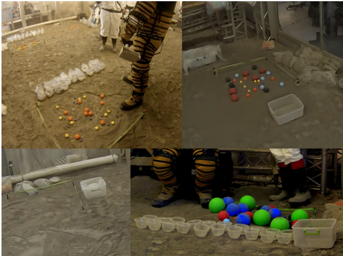
Figure 39. Experimental set-ups, top-left rotating clock-wise; scoop target test, rake test, tongs test {Credit: NASA-JSC: Larry K. Dungan}, scoop regolith test.
