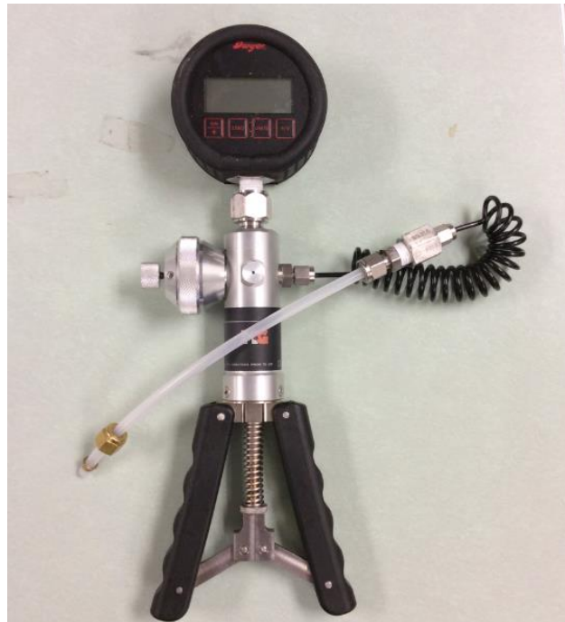
Figure 41: The combination of DPG-107 Dwyer digital pressure gauge and A T-970 Ametek pneumatic hand air calibration pump
