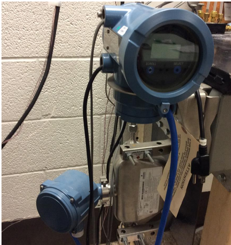
Figure 33: Mass flow meter
