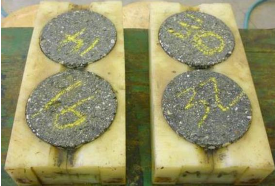
Figure 3: Placing specimens in the molds for running in APA
