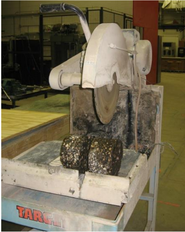
Figure 2: The concrete saw used in sizing the specimens to APA height requirements.
