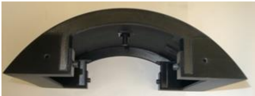
Figure 7. The assembled 0.4064 meter cylindrical leading edge tip.
