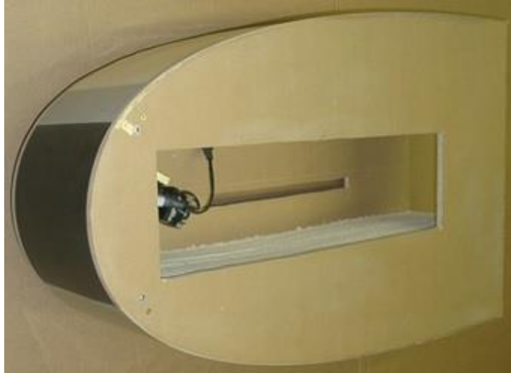
Figure 6. The 0.4064 meter cylindrical leading edge vane.
