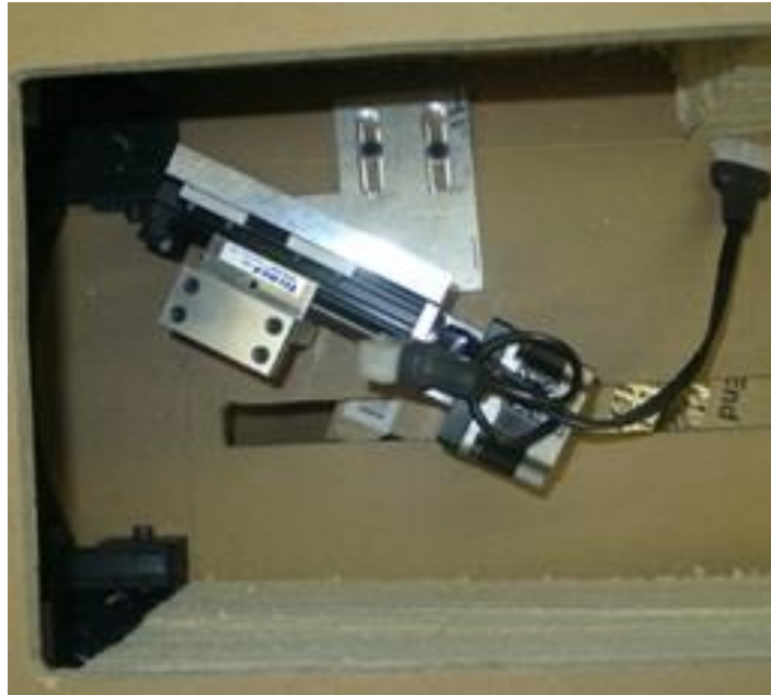
Figure 15. Traversing equipment mounted in test apparatus.
